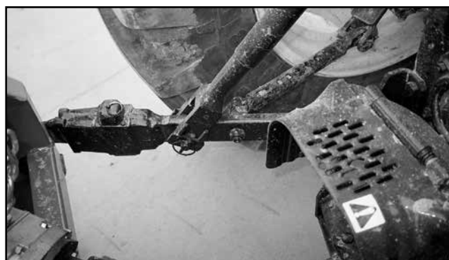
Fig. 13 —Sway anchor pin (typical)
