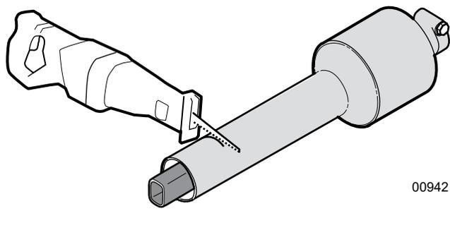
Fig. 5 – Cut plastic tube at the mark
