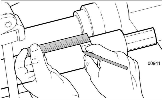
Fig. 4 – Place mark to cut plastic tube
