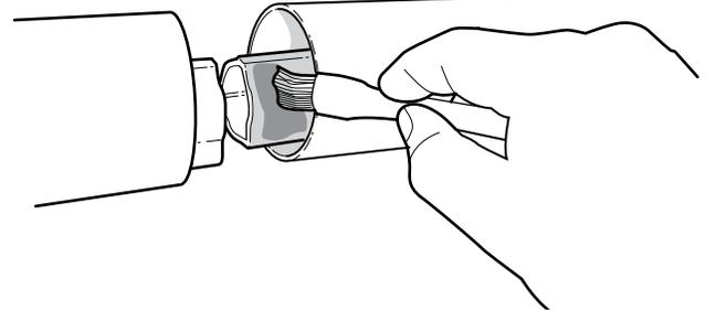
Fig. 7 – Grease the inner tube
