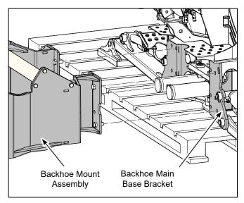
The Subframe should remain on your backhoe and not be removed. Check that the lift arms move freely with the Subframe installed.
