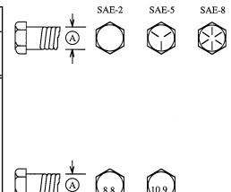
Torque figures indicated above are valid for non-greased or non-oiled threads and heads unless otherwise specified. Therefore, do not grease or oil bolts or caps crews unless otherwise specified in this manual. When using locking elements, increase torque values by 5%.
