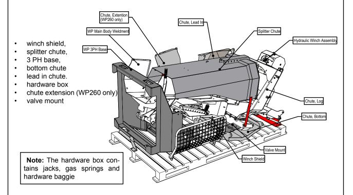
6. After removing the components from the skid, fasten the splitter weldment to the 3 PH adaptor. Swivel the splitter weldment over (as shown) to line up the 9 remaining bolt holes. Insert the bolts and nuts and fasten securely.
