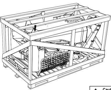
**Caution:** Heavy or bulky parts: prevent potential injury ask for help when lifting or moving heavy, bulky parts.
