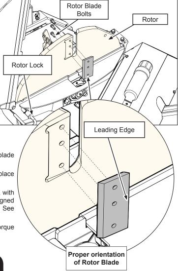
**Rotor Blade:** depending on your model the rotor blade may have 4 mounting holes. The removal replacement procedure is the same for both.
