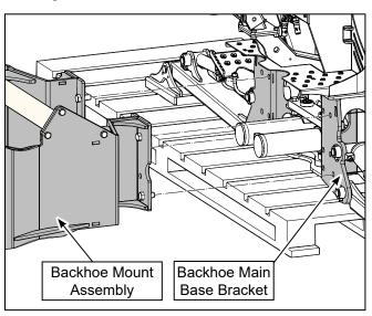
The subframe should remain on your backhoe and not be removed. Check that the lift arms move freely with the subframe installed.
