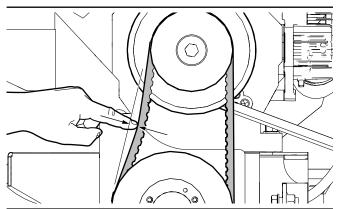
Fig. 61 – Drive belt tension
