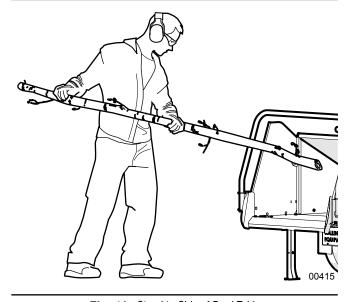
Fig. 41 – Stand to Side of Feed Table
