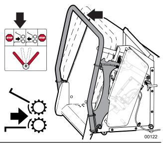
Fig. 40 - Forward Feed Position
