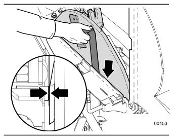
Fig. 69 - Checking ledger knife clearance
