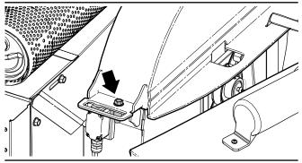
Fig. 42 - Rotor Housing Flange Bolt
