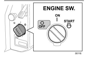
Fig. 9-Engine Start Switch
