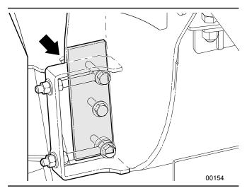
Fig. 68-Ledger knife inside lower rotor housing
