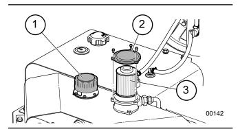
Fig. 56-Hydraulic Oil Filter Element
