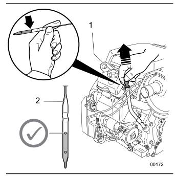
Fig. 32-Checking Engine Oil Level
