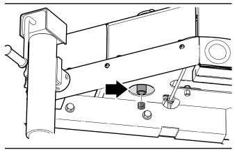
Fig. 53 - Hydraulic Tank Drain Plug
