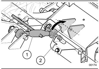
Fig. 44 - Connect Toplink to Bridge
