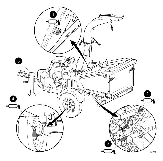
Fig. 50 - Grease Points - 50 Hours of Operation or Annually
