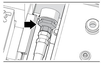
Fig. 54 - Suction Strainer on Hydraulic Tank
