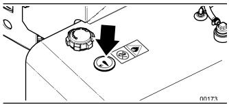
Fig. 30 - Fuel Level Gauge
