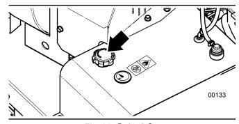
Fig. 31 - Fuel tank Cap
