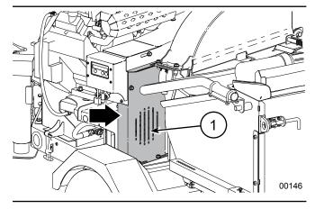
Fig. 58-Lower drive belt shield
