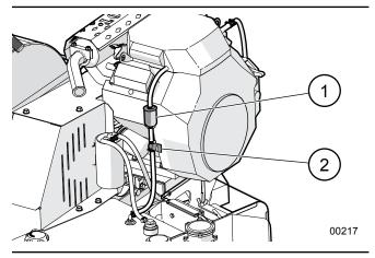
Fig. 74-Engine Fuel Filter
