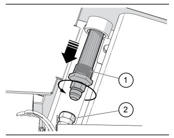
Fig. 55 – Suction Strainer on back of Hydraulic Tank
