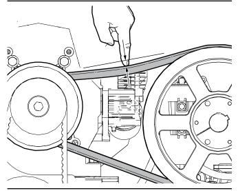
Fig. 65 - Rotor drive belt tension
