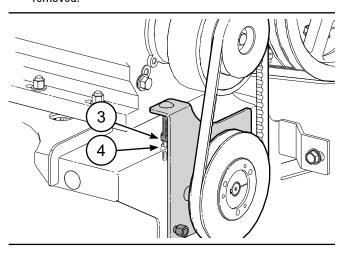
Fig. 60 - Belt Tension Adjuster
