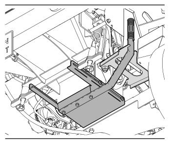
Fig. 29 - View of Clean-out Tray from Underside of Chipper
