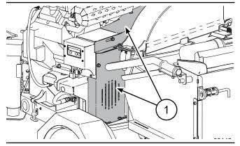
Fig. 62-Upper and lower drive belt shields
