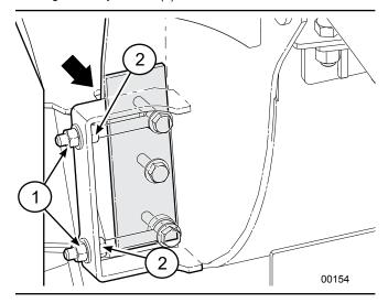
Fig. 70 - Adjusting ledger knife clearance
