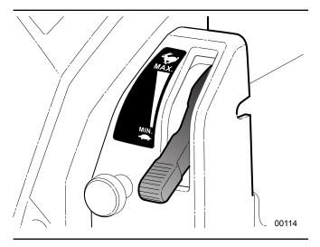
Fig. 7-Throttle Lever
