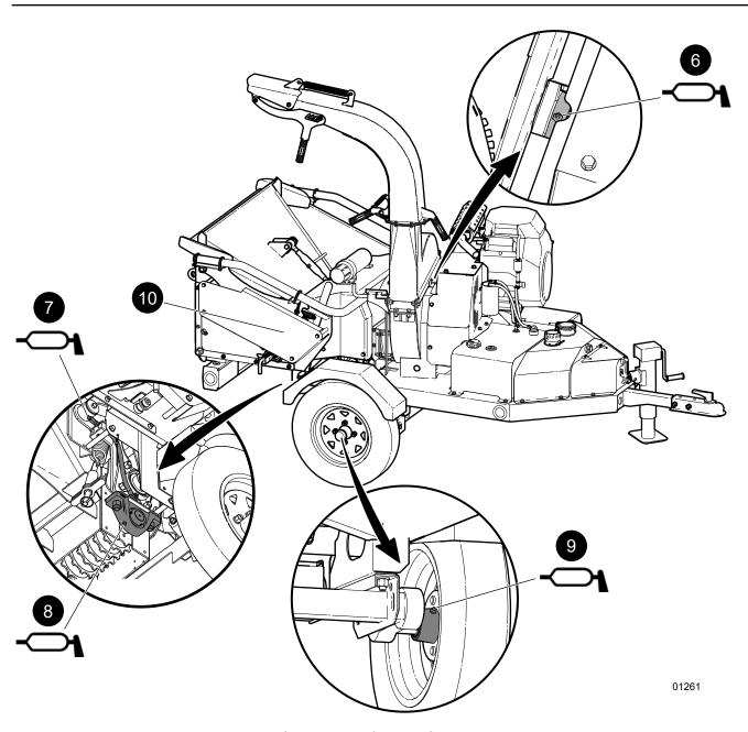
Fig. 51 – Grease Points – 50 Hours of Operation or Annually
