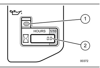
Fig. 10 - Engine Hours and Oil Level Alert
