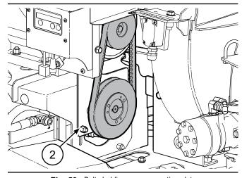
Fig. 59 – Bolts holding pump mounting plate
