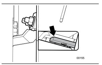
Fig. 72-View of Ledger Knife from underside of Chipper
