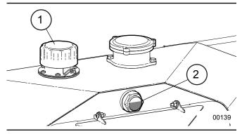
Fig. 33-Hydraulic Tank Oil Level Check
