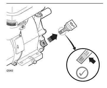
Figure 11 - Check the engine oil level
