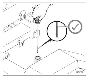
Figure 14-Hydraulic tank fluid level dipstick
