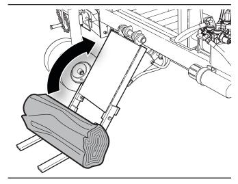
Figure 18 - Lift the log lifter shelf
