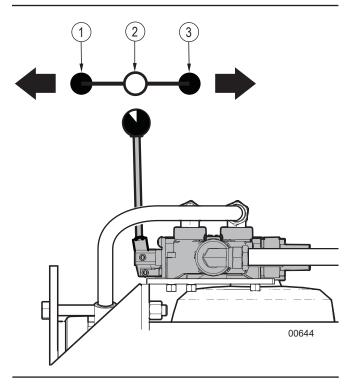
Figure 9-Splitter-control valve
