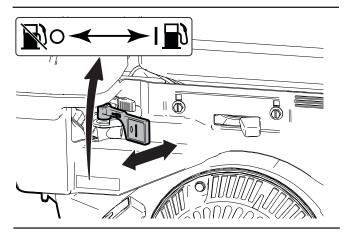
Figure 5-Engine fuel shutoff
