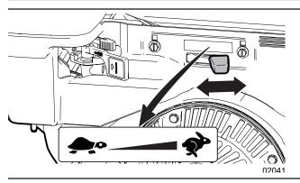
Figure 4-Engine throttle control
