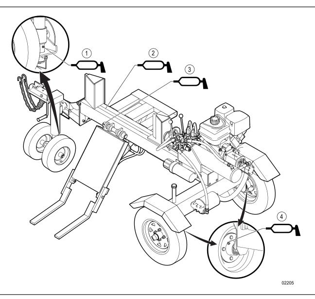
Figure 23 – Grease fitting and hinge/pivot point locations
