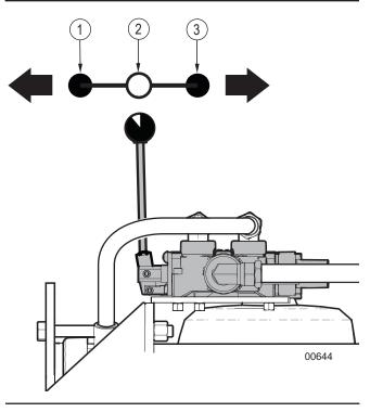
Figure 20 - Splitter-control valve
