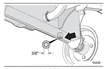
Figure 24-Hydraulic fluid reservoir drain plug
