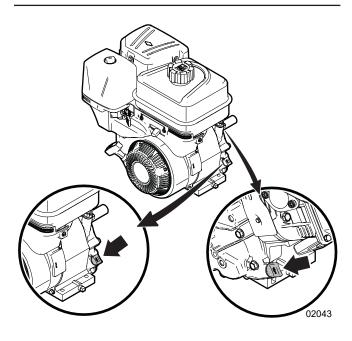
Figure 12-Engine oil-fill locations
