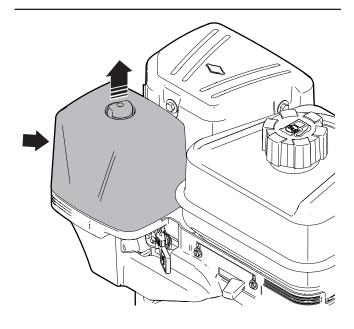
Figure 26-Remove the air filter
