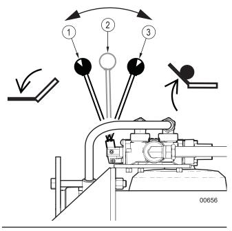
Figure 10-Log lifter shelf control valve
