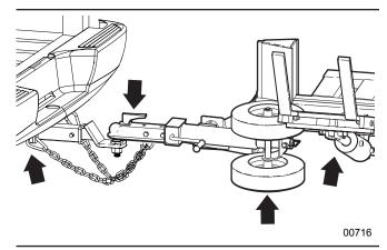
Figure 22 - Attach to a tow vehicle
