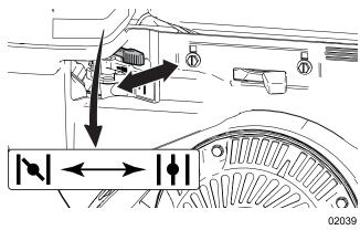
Figure 6-Engine choke control
