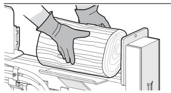
Figure 19-Correct log placement
