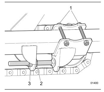
Figure 26 - Apron-chain Adjustment
