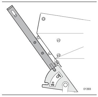
Figure 18 - Ground Drive Disengaged
