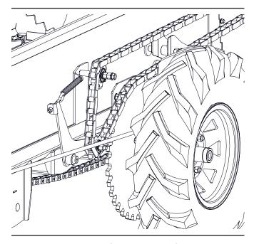
Figure 25 – Ground-drive Roller Chain
