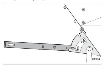
Figure 20 - Ground Drive Engaged
