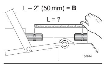
Figure 9-Measurement B
