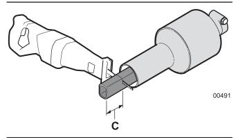
Figure 11 - Cut Off Length C from Both PTO Shaft Halves
