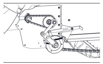
Figure 24 - Roller Chain and Apron Chain
