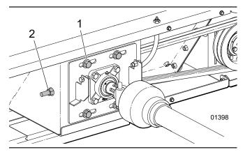
Figure 31 - Tensioning a Drive Belt
