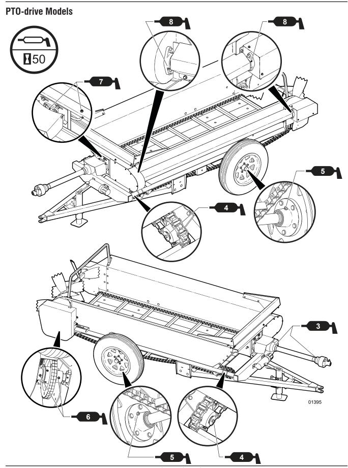
Figure 22-PTO-drive 50-hour Grease Points
