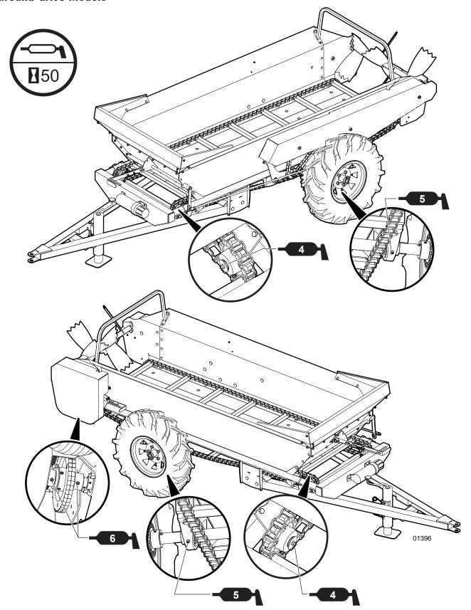
Figure 23 - Ground-drive 50-hour Grease Points
