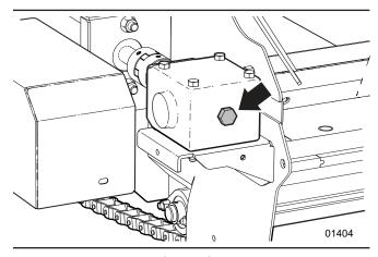
Figure 29 - Gearbox Oil-reservoir Plug
