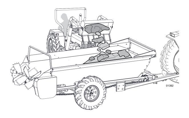
Figure 16-Load the Manure Spreader
