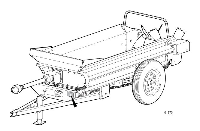
Figure 1 – Serial Number Plate Location (Typical)
