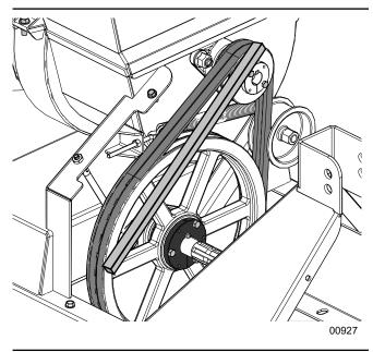
Fig. 55 - Sheave Alignment (BXM32 shown)
