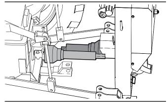
Fig. 10-Lift shaft ends up parallel
