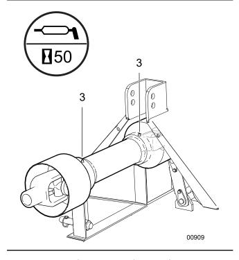
**Fig. 35 –** Grease Points – 50 Hours of Operation
