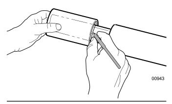
Fig. 14-Marking steel tube.
