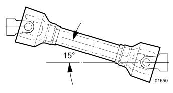
Fig. 21 – Driveshaft Alignment
