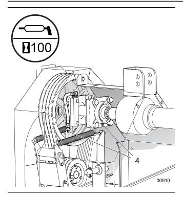
Fig. 38 - BXM42 Rotor PTO Bearings
