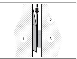
Fig. 47 - Checking ledger knife clearance
