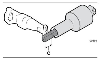
Fig. 19 - Cut off the Length C from both PTO Shaft halves
