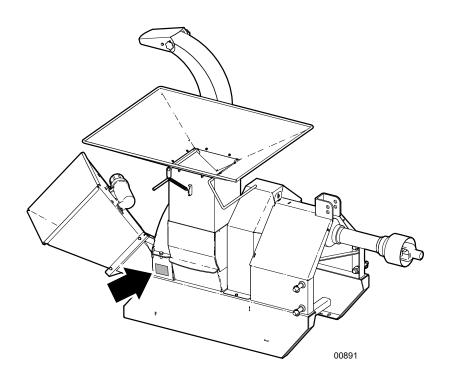
Fig. 1 – Serial Number Plate Location (Typical)
