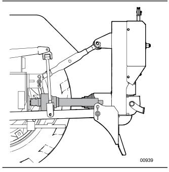
Fig. 9-Input shaft and output shaft
