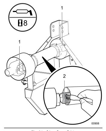
Fig. 34 - 8-hour Grease Points
