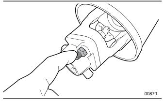
Fig. 41-PTO Shear Bolt
