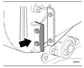
Fig. 45-Ledger knife on lower rotor housing
