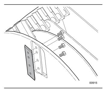
Fig. 43 - Changing rotor blade
