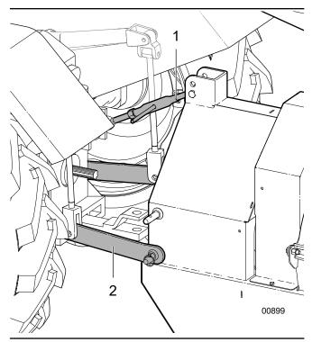
Fig. 8-Three-point Hitch Connected
