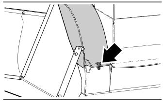
Fig. 30—Rotor Housing Bolt
