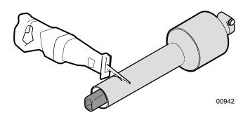
Fig. 13 - Cut plastic tube at the mark
