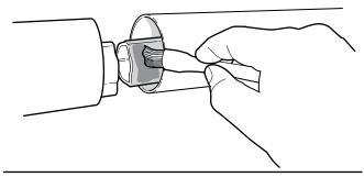
Fig. 15-Grease the inner tube
