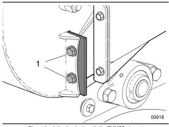
Fig. 48 - Adjusting Ledger Knife (BXM32 shown)
