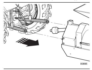
Fig. 7 - Back up in line with the chipper
