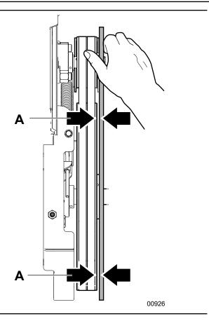
Fig. 56-Top View of Sheave Alignment (BXM32 shown)
