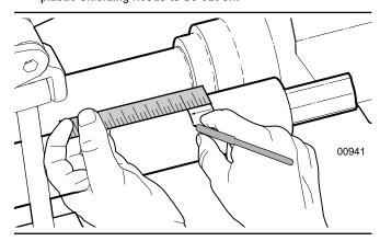
Fig. 12-Place mark to cut plastic tube
