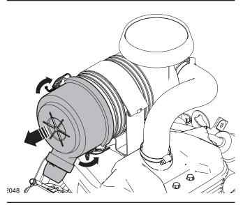
Figure 24 - Remove the air-filter cover
