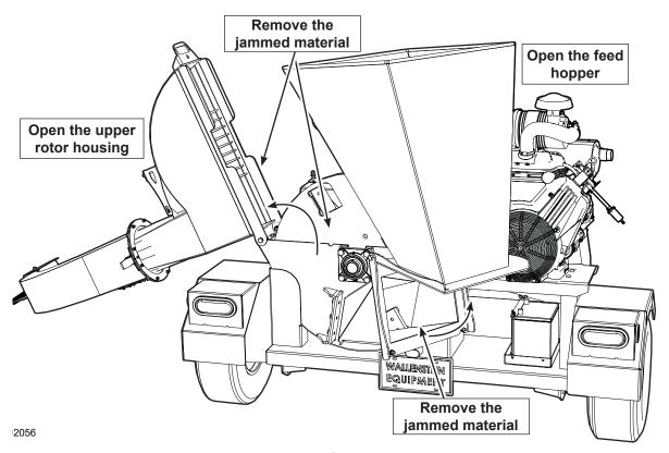
Figure 18-Clear a severe jam
