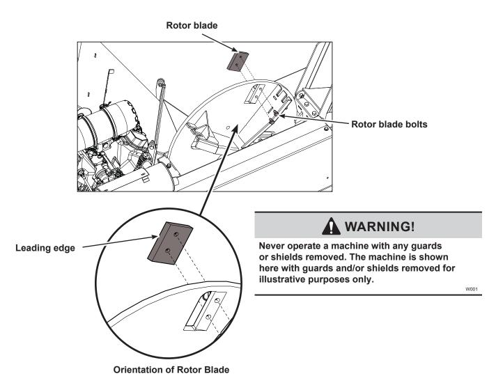
Figure 28 - Rotor blade
