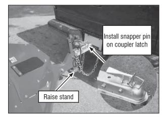
Figure 11 – Attaching to a tow vehicle
