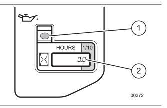
Figure 9-Engine Hours and Oil Level Alert
