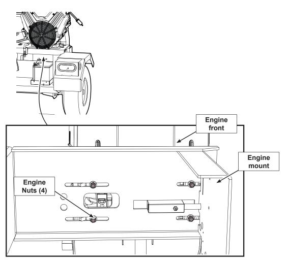
Figure 25 - Bottom view of the engine mount
