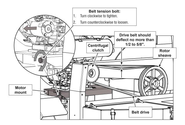
Figure 26 - Check the drive belt tension
