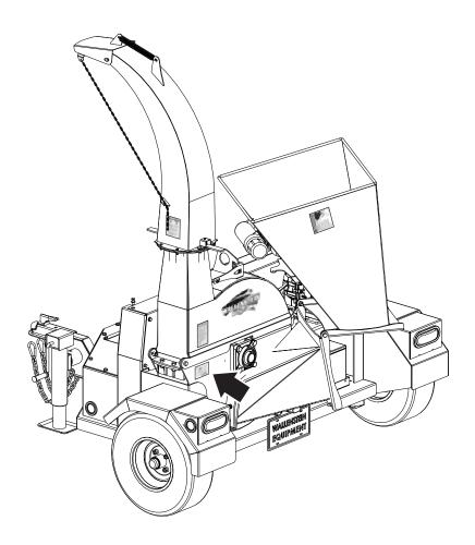
Figure 1 – Serial Number Location (typical)
