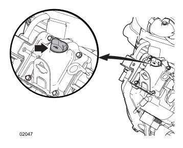
Figure 16 – Engine oil-fill location
