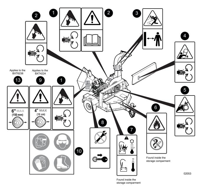
Figure 2-Safety signs on the machine
