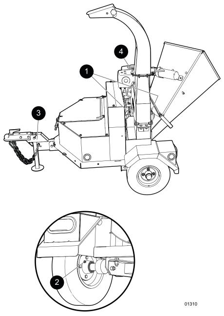
Figure 23 – Grease points (typical)
