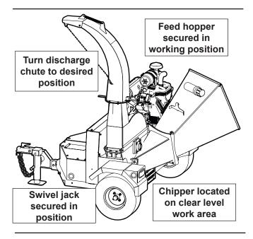
Figure 14-Machine setup
