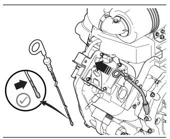
Figure 15-Check the engine oil level
