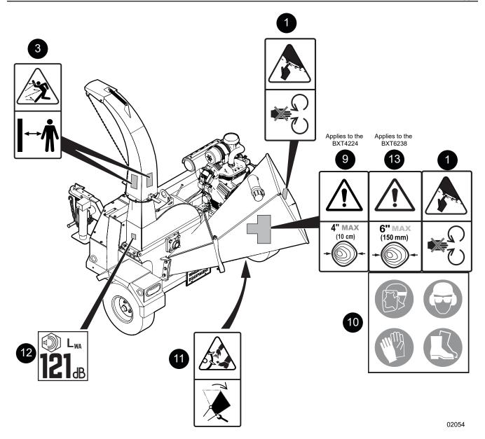
Figure 3 – Safety Signs on the machine
