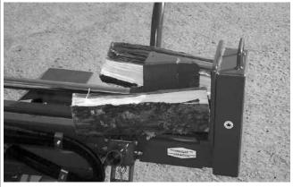
Fig. 17 HORIZONTAL SPLITTING
