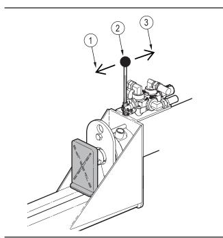
Figure 6-Splitter-control valve
