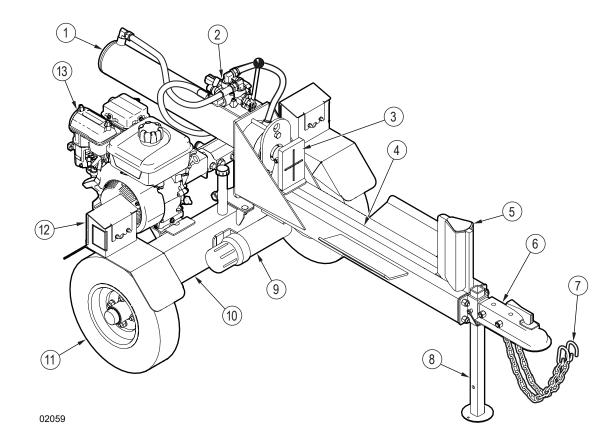
Figure 2-WX520, WX520T, and WX520L log splitter components
