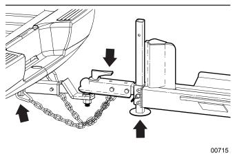
Figure 14–Align the ball hitch
