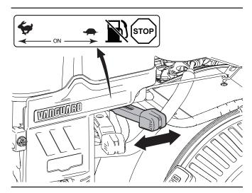
Figure 3-Engine throttle control and fuel shutoff
