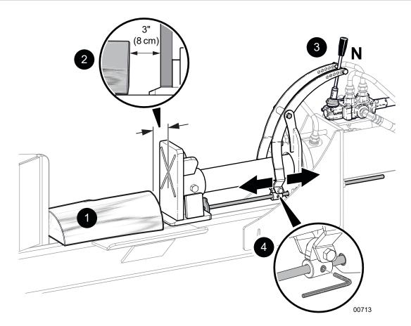
Figure 15-Adjust the stroke limiter
