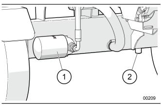
Figure 18–Hydraulic Filter
