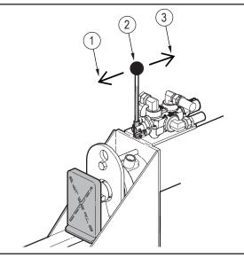
Figure 13-Splitter-control valve
