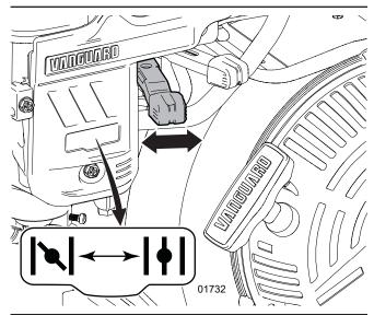
Figure 4-Engine choke control
