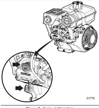
Figure 8–Engine oil-fill locations
