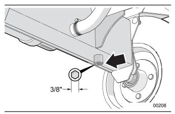
Figure 17 – Hydraulic Tank Drain Plug
