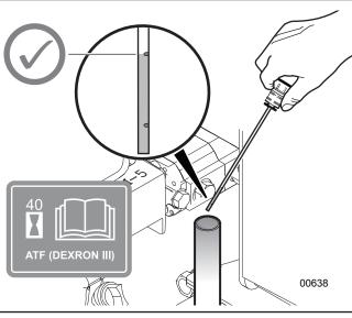
Figure 9-Hydraulic tank fluid level dipstick
