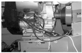
a. Engine Mounting Bolts b. Adjusting Bolt Fig. 53 BELT DRIVE SYSTEM
