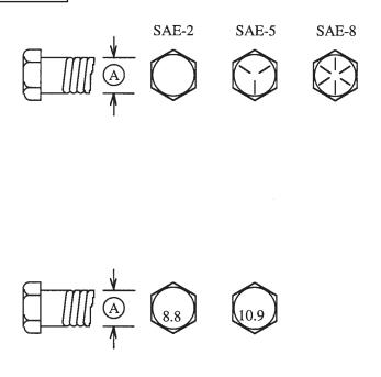
Torque figures indicated above are valid for non-greased or non-oiled threads and heads unless otherwise specified. Therefore, do not grease or oil bolts or capscrews unless otherwise specified in this manual. When using locking elements, increase torque values by 5%.
