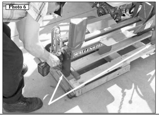
7. Suspend splitter slightly off skid and remove the shipping brackets from splitter. *Photo* 7
