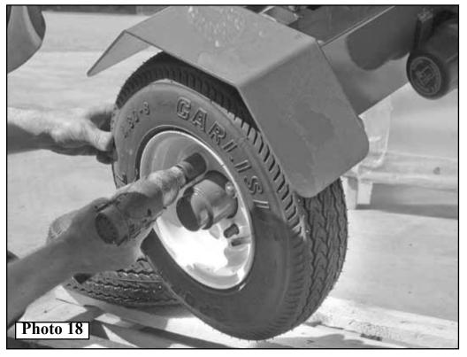
17. Install one (1) 4.80-8 LRB SportTrail 3-3/4 Solid, Left Side Tire and secure with four (4) Lug Nut 1/2NF. *Photo 19*
