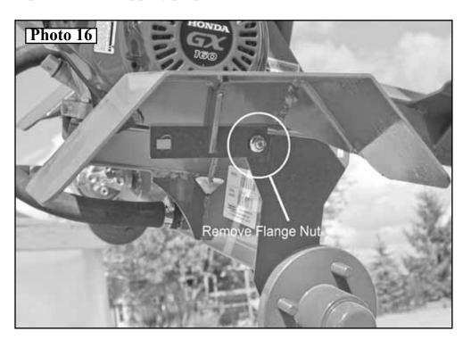
Reassemble the fender back to the right side moving it forward and securing it with two (2) 3/8 x 3/4 Carriage Bolts and two (2) 3/8" Flange Nuts. *Photo 17*
