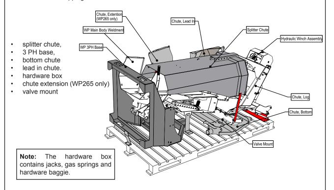
6. After removing the components from the skid, fasten the splitter weldment to the 3 PH adaptor. Swivel the splitter weldment over (as shown) to line up the 9 remaining bolt holes. Insert the bolts and nuts and fasten securely.
