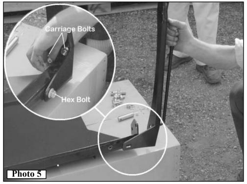
5. Install the End Gate assembly to the spreader attaching it at the pin locations on the previously installed End Gate Pivot Bases *Photo* 6
