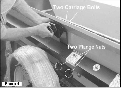
4. Loosley attach the L.H & R.H End Gate Swing Arms to each side of the End Gate using (2) Carriage Bolt 1/2NC x 1, (1) Hex Bolt, 1/2NC x 1 & (3) Hex Lock Nut, 1/2NC. Photo 5
