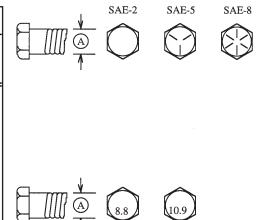
Torque figures indicated above are valid for non-greased or non-oiled threads and heads unless otherwise specified. Therefore, do not grease or oil bolts or caps crews unless otherwise specified in this manual. When using locking elements, increase torque values by 5%.
