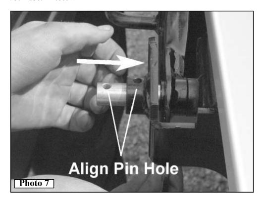
7. Secure with (1) Hex Bolt 1/4NC x 1-1/2 & (1) Hex Locknut, 1/4NC. *Photo 8* Repeat on other side.
