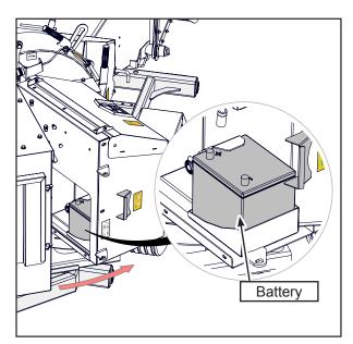
WARNING: frozen batteries can explode and result in death or serious injury. DO NOT charge a frozen battery. Let battery thaw before charging.
