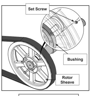
Note: movement of the sheave may occur when tightening the bushing, some allowance for movement may be required.
