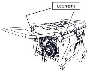
Do not lift entire generator by folding handle. Folding handle is not intended for motorized transport of generator.
