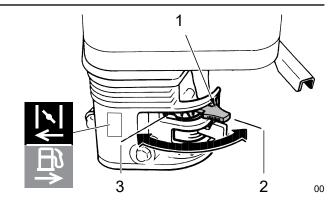
Fig. 18-Choke Lever
