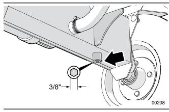
Fig. 29 - Hydraulic Tank Drain Plug
