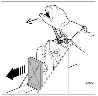
Fig. 12 - Extend Push Block to split Wood
