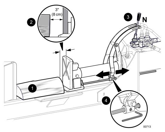
Fig. 27 - Stroke Limiter Adjustment
