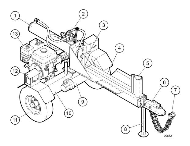
Fig. 3-WX520, WX520T and WX520L Wood Splitter Components
