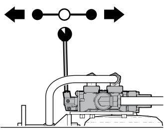
Fig. 24-Hydraulic Control Valve Positions
