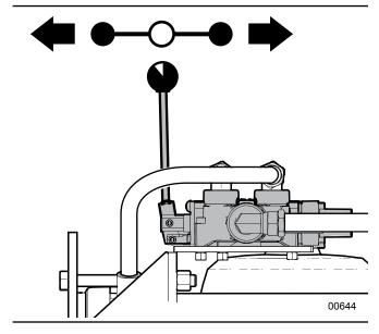
Fig. 10-Splitter Control Valve
