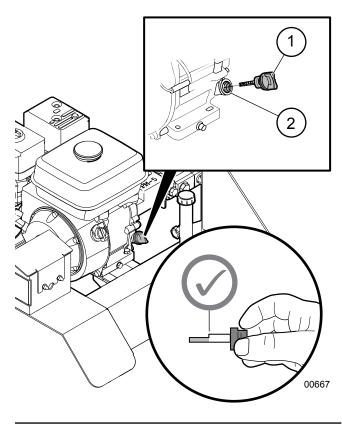
Fig. 14-Engine Oil Level check
