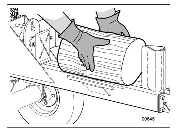
Fig. 23-Correct Log Placement
