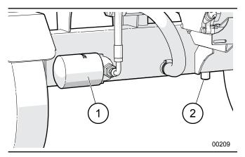
Fig. 30 - Hydraulic Filter
