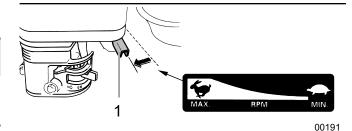
Fig. 19 - Engine Throttle
