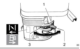
Fig. 9-Choke Lever
