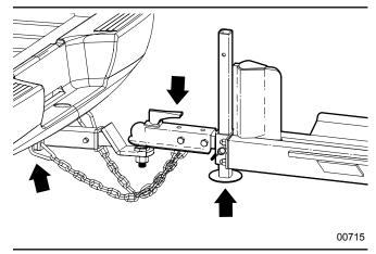
Fig. 26-Ball Hitch Aligned
