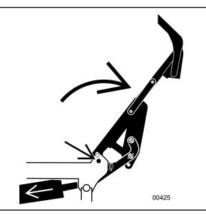
Fig. 22-Line up Holes in the Live Deck
