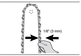
Fig. 84-Saw Chain Tension
