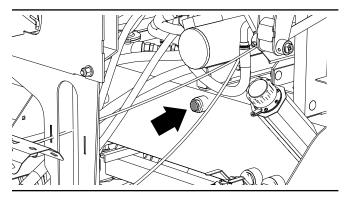
Fig. 35-Hydraulic Tank Oil Level Check
