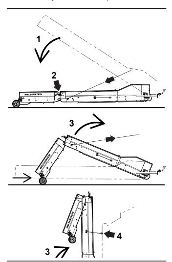
Fig. 62-Folding up 12 ft (3.6 m) Conveyor
