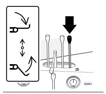
Fig. 59-Log Lifter Control Valve Lever
