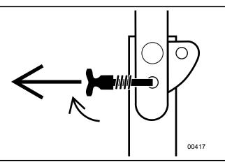
Fig. 16-Pull and lock out Pins on Both Sides
