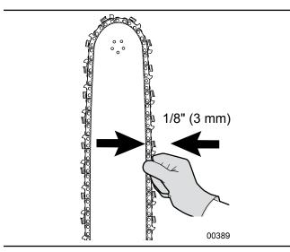
Fig. 38-Check Saw Chain Tension
