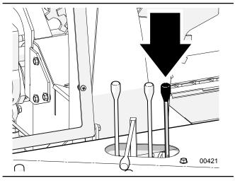
Fig. 14-Log Lifter Shelf Control Valve Lever
