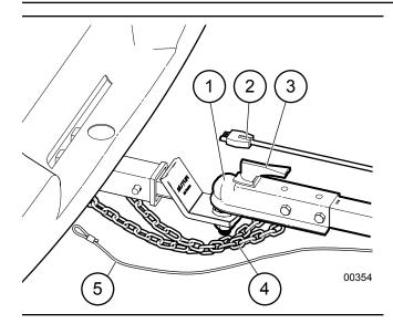
Fig. 66 - Attaching to a Tow Vehicle
