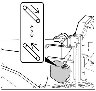
Fig. 56-Conveyor Control Lever
