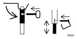
Fig. 20 - Set up Support Legs under the Live Deck
