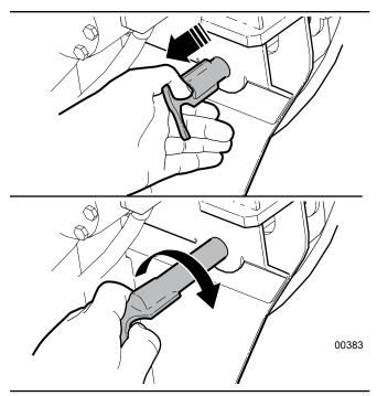
Fig. 15-Live Deck Locking Pins
