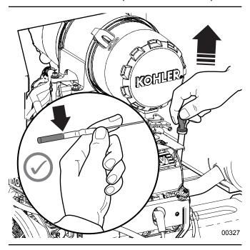
Fig. 34-Checking Engine Oil Level
