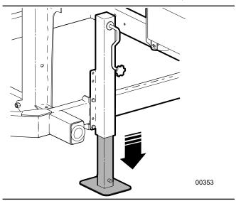
Fig. 8-Front Crank Jack
