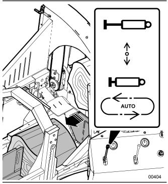
Fig. 55-Splitter Control Lever
