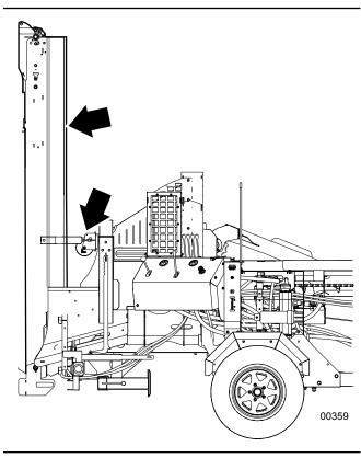
Fig. 61-8 ft (2.4 m) Conveyor in Transport Position
