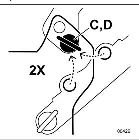
Fig. 23-Install Pins C and D
