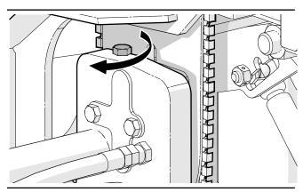
Fig. 83 – Turn Adjusting Screw Clockwise to Increase Chain Tension
