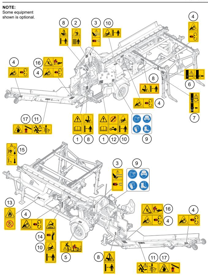
Fig. 3 - Safety Decal Placement
