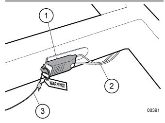
Fig. 67 - Trailer Breakaway Switch
