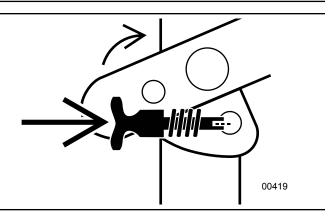
Fig. 17-Release Locking Pins
