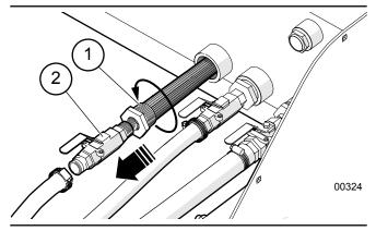
Fig. 72-Suction Strainer Removal
