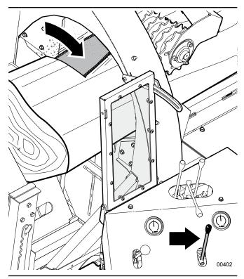
Fig. 50 - Cutting the Log
