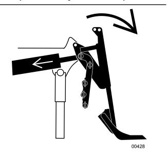
Fig. 25-Retract the Log Lifter Cylinder
