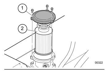
Fig. 74-Hydraulic Oil Filter Element
