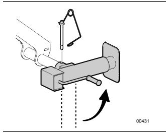
Fig. 64-Rotate Crank jacks
