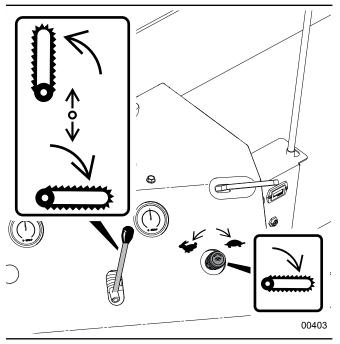
Fig. 49 - Saw Control Lever and Feed Rate Control
