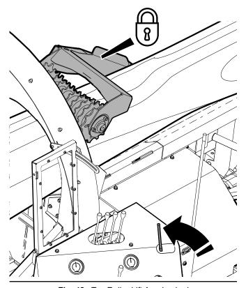
Fig. 48 - Top Roller Lift Arm Locked
