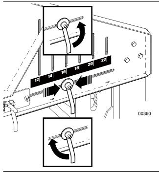
Fig. 29-Log Stop Guide Lock Handle
