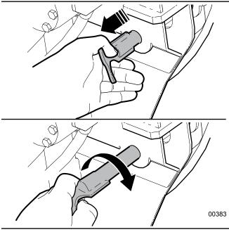
Fig. 10-Live Deck Locking Pins
