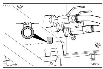
Fig. 70 - Hydraulic Tank Drain Plug
