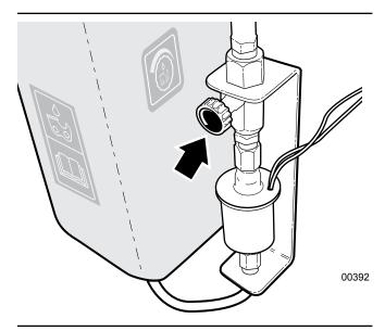
Fig. 53-Bar Oil Flow Control
