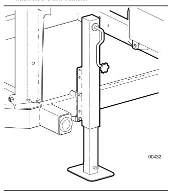
Fig. 65-Front Crank Jack
