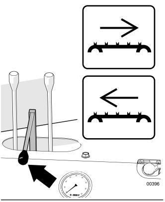
Fig. 42-Infeed Conveyor Control Valve
