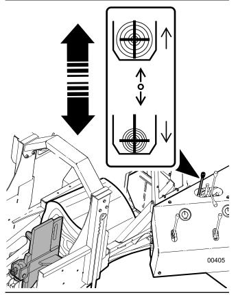
Fig. 54-Adjust Wedge Height
