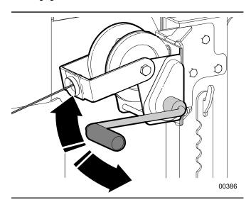
Fig. 92-Conveyor Hand Winch
