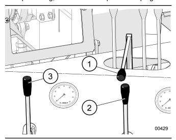
Fig. 39-Infeed Conveyor, Saw Cut, and Splitter Controls
