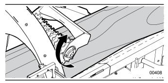
Fig. 51 - Powered Top Roller
