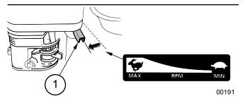
Fig. 21 - Engine Throttle
