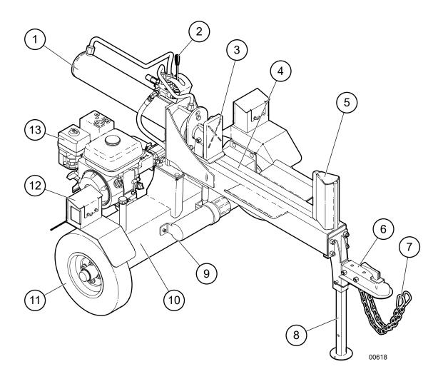
Fig. 3-WXR720, WXR720L Wood Splitter Components
