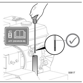
Fig. 13-Hydraulic Tank Oil Level Dipstick
