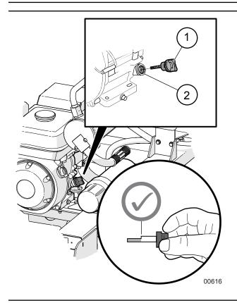
Fig. 12-Engine Oil Level check
