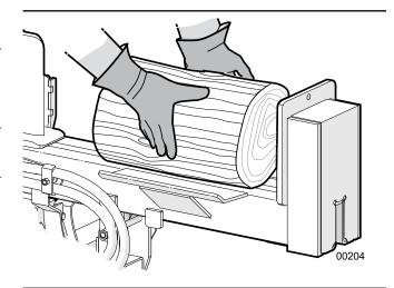
Fig. 25-Correct Log Placement
