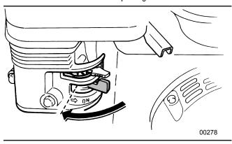
Fig. 30 - Fuel Valve OFF
