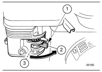
Fig. 8-Fuel Valve Lever
