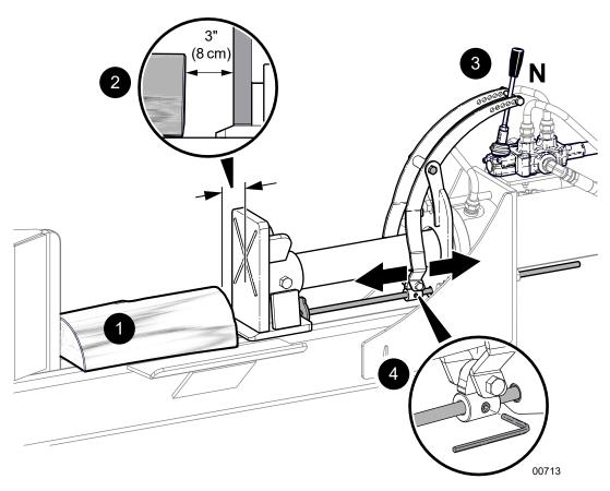
Fig. 32-Stroke Limiter Adjustment
