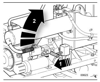
Fig. 18-Rotate Splitter to Vertical
