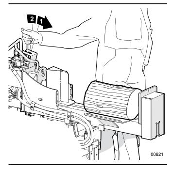
Fig. 27-High Speed (2), High Power (1)
