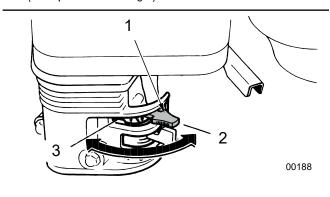
Fig. 20-Choke Lever
