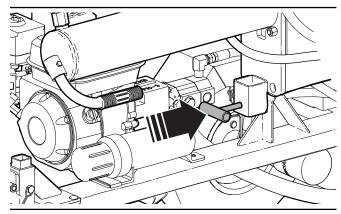
Fig. 29-Lock Pin Fully Engaged on WXR740 Series
