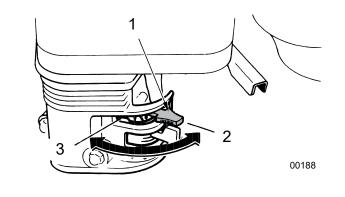
Fig. 7-Choke Lever
