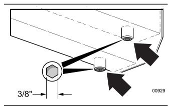
Fig. 34-Hydraulic Tank Drain Plugs
