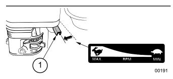
Fig. 9-Throttle Lever Positions
