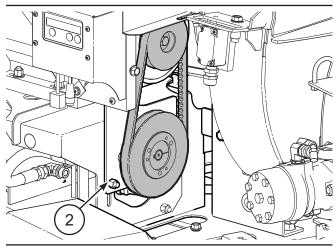
Fig. 58-Bolts holding pump mounting plate
