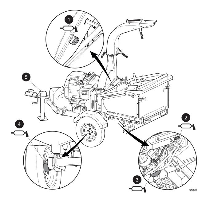
Fig. 49-Grease Points - 50 Hours of Operation or Annually
