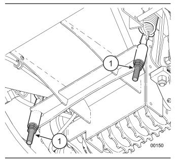
Fig. 65-Upper feed roller tensioner (US model shown)
