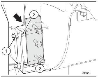
Fig. 69-Adjusting ledger knife clearance
