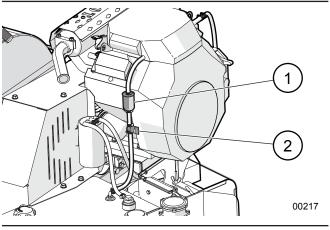
Fig. 73–Engine Fuel Filter
