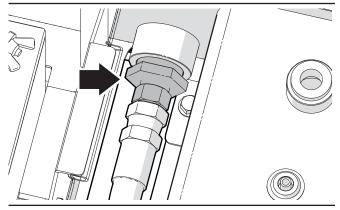
Fig. 53-Suction Strainer on Hydraulic Tank
