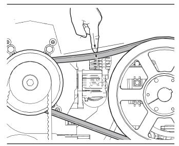
Fig. 64-Rotor drive belt tension
