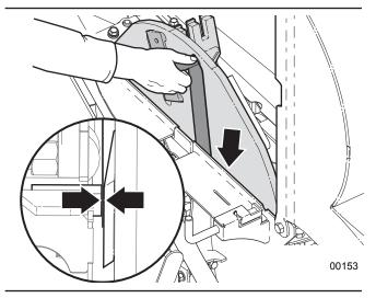
Fig. 68 – Checking ledger knife clearance
