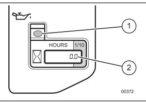
Fig. 10-Engine Hours and Oil Level Alert
