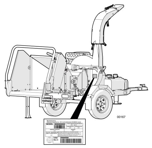
Fig. 1-Serial Number Plate Location
