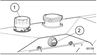
Fig. 32-Hydraulic Tank Fluid Level Check
