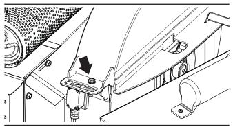
Fig. 41 – Rotor Housing Flange Bolt
