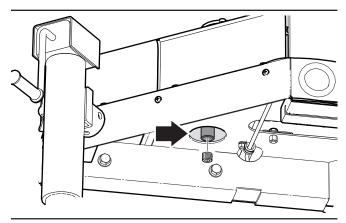
Fig. 52-Hydraulic Tank Drain Plug
