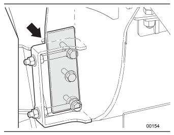
Fig. 67-Ledger knife inside lower rotor housing
