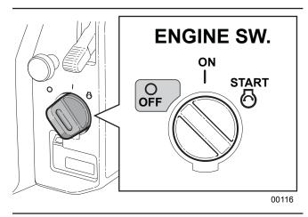
Fig. 9-Engine Start Switch
