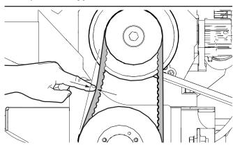
Fig. 60-Drive belt tension
