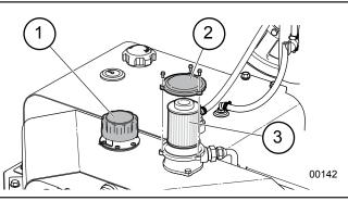
Fig. 55-Hydraulic Fluid Filter Element
