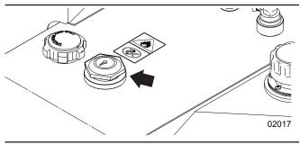
Fig. 29-Fuel Level Gauge
