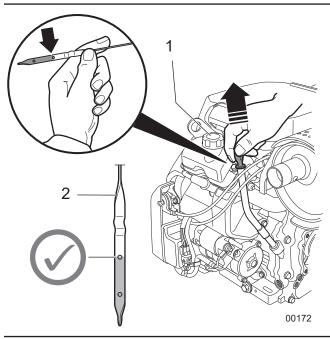
Fig. 31 – Checking Engine Oil Level
