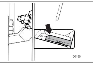
Fig. 71-View of Ledger Knife from underside of Chipper
