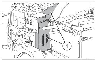
Fig. 61 – Upper and lower drive belt shields
