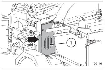
Fig. 57 – Lower drive belt shield
