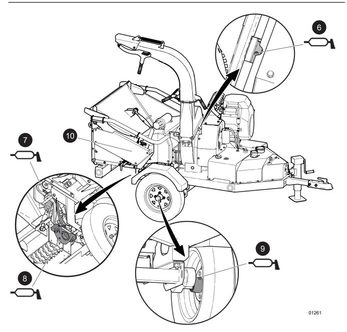
Fig. 50 - Grease Points - 50 Hours of Operation or Annually
