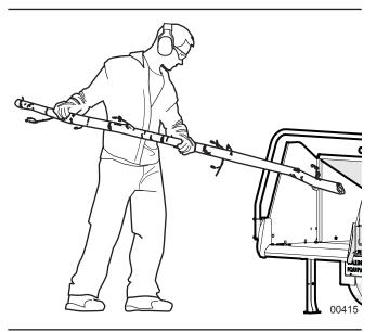
Fig. 40-Stand to Side of Feed Table
