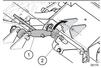
Fig. 43-Connect Toplink to Bridge
