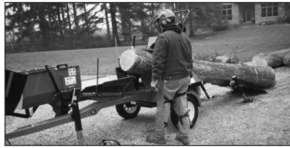
Winching to Cutting Guide
