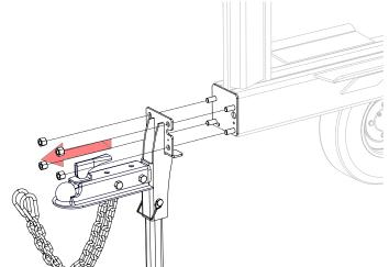
3. With a helper, position the shelf base on to the four mounting bolts. While your helper holds the shelf in place, fit the stand/hitch assembly over the shelf base.
