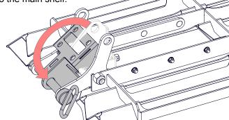
2. Support the wood splitter so the stand is not supporting any weight, then remove the stand/hitch assembly. Discard the nuts.
