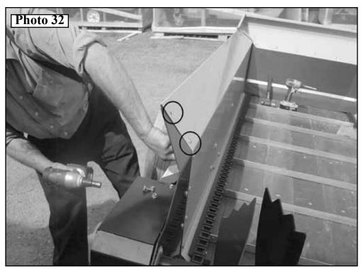
33. Remove (2) Carriage Bolt, 5/16NC x 3/4 & (2) Flange Nut, 5/16NC at rear of spreader on Right Hand Side Panel (to mount the Cross Bar). *Photo 33*
