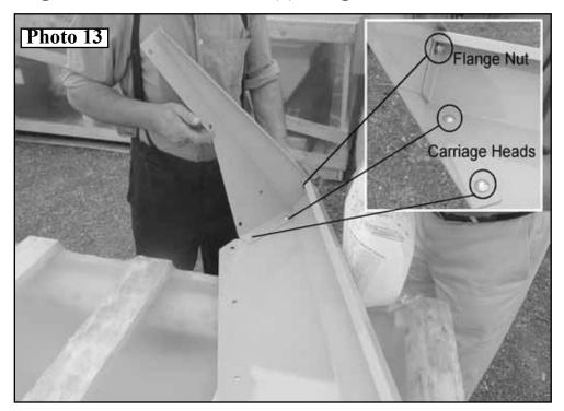
13. Take the Splash Guard Assembly to the front of the spreader and place into position. *Photo 14*
