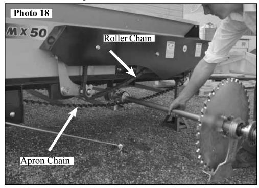
18. Temporarily align the Ground Drive Axle Sprocket with the Roller Chain above. *Photo 19*
