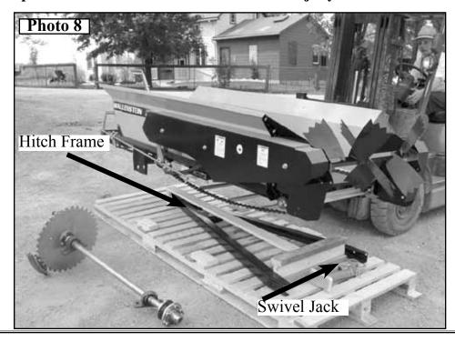
8. Carefully set the spreader down and support with jacks at each of four corners on the lower frame. *Photo 9*
