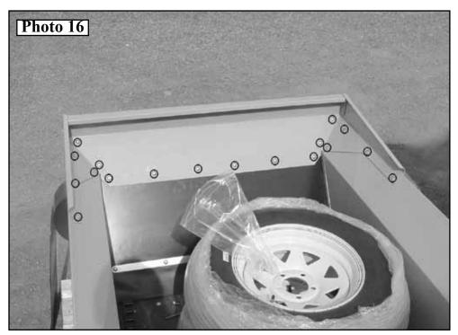
16. Locate Engagement Rod running down right hand side of spreader. Snip tie wrap securing it to roller chain for shipping purposes. Swivel out of way. *Photo 17*
