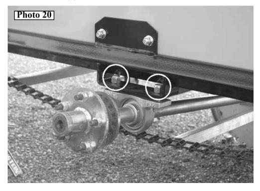
20. Loosely secure the axle to the DRIVE side of the spreader with (2) **Hex Bolt, 5/8NC** x 1-1/2 & (2) **Hex Lock Nut, 5/8NC**. *Photo 21*
