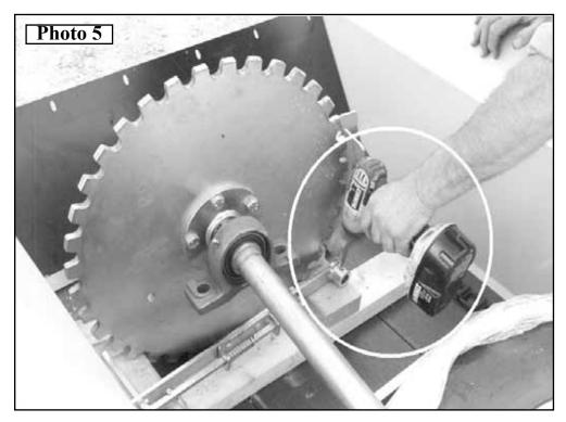
5. Remove the **Hex Bolt 5/16NC x 2 & Hex Lock Nut 5/16NC** temporarily mounted at the Drive Engagement Connection Rod (for your convenience. Inset A). Use this hardware to mount and secure the Engagement Handle Assembly. *Photo 6*
