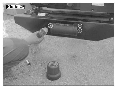
26. Remove the (2) Carriage Bolt, 1/2NC x 1-1/2 & (2) Hex Lock Nut, 1/2NC, from the location on the Hitch where it will be attached to the spreader. This hardware is shipped mounted here for your convenience. *Photo 26*
