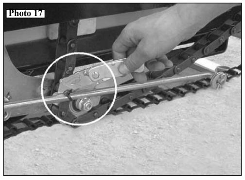
17. Enlisting the help of a second pair of hands, pass the Ground Drive Axle Assembly under the spreader (from right side), to a second person on the left side.
