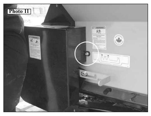
11. Secure the Apron Drive Shield with (2) two **Flange Bolt 5/16NC x 3/4** to the inside. *Photo 12*
