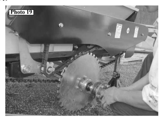
19. Loosely secure the axle to the bracket on the left side of the spreader with (2) Hex Bolt, 5/8NC x 1-1/2 & (2) Hex Lock Nut, 5/8NC. Photo 20
