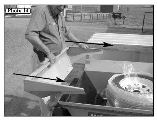
14. Loosely install (14) Carriage Bolts, 5/16NC x 5/8 and (14) Flange Nut, 5/16NC, to the Splash Guard assembly, working from one side to the other. *Photo 15*
