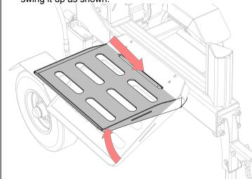
2. Have some one hold the shelf in position and slide in the clamping plate under the wing and bolt to the shelf as shown, using the carriage bolts and lock nuts supplied.
