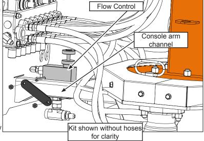
and install the bolts and bracket, and tighten up with the nuts.
