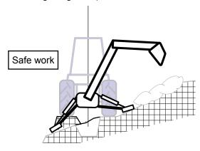
for greatest stability, swing the boom upside the slope, but if swing downside is required, do so with extreme caution and swing only as far as necessary to dump the bucket. When excavating be aware:
