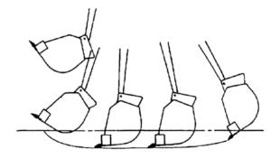
**NOTE:** Be sure the dipper and bucket angles are set so that the heel of the bucket does not hit the bottom of the hole.
