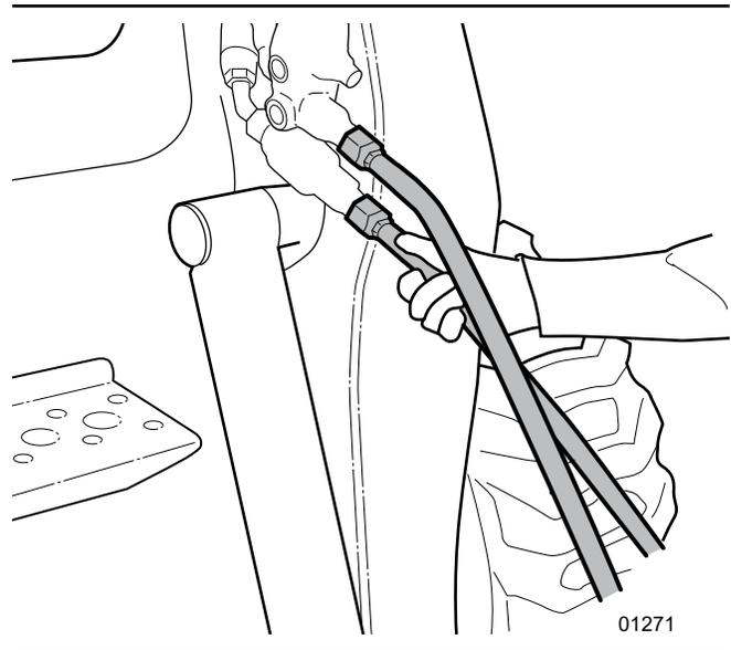
Fig. 4—Connect pressure and return hoses
