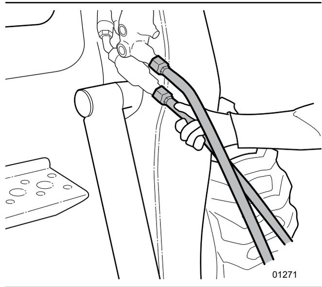
Fig. 4—Connect pressure and return hoses
