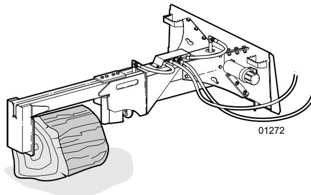
Fig. 6—Positioning splitter over the wood block
