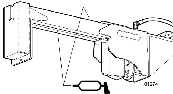
Fig. 8—Greasing Splitter Bed Slide
