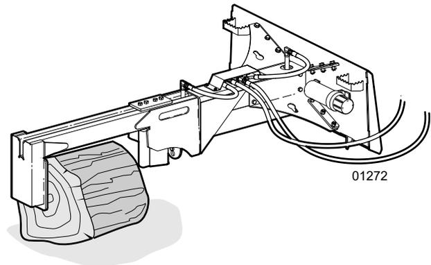
Fig. 6 – Positioning splitter over the wood block
