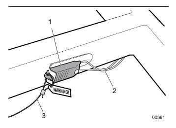
Fig. 73 - Trailer Breakaway Switch
