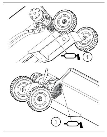
Fig. 94-12 ft Conveyor Grease Points
