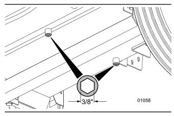
Fig. 77 - Hydraulic Tank Drain Plug
