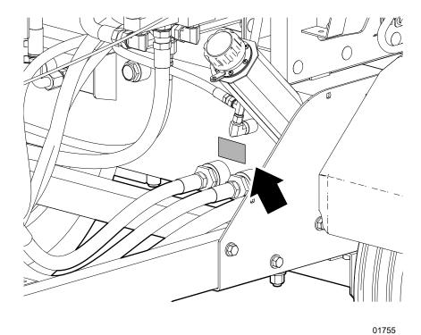
Fig. 1 - Serial Number Plate Location
