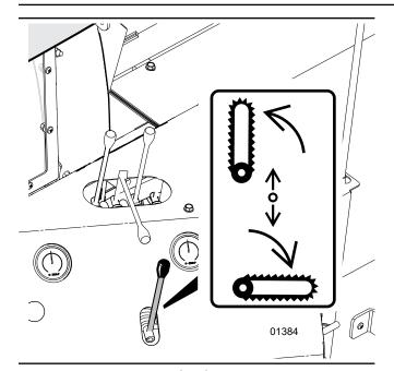
Fig. 54-Saw Control Lever
