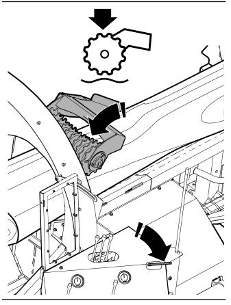
Fig. 51 - Top Roller Lift Arm Clamped Down on Log
