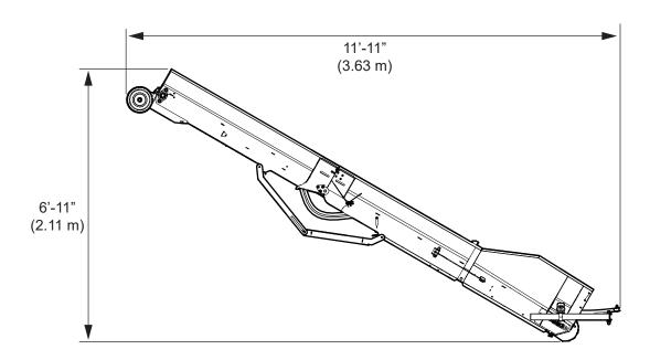
Fig. 102-12 ft Conveyor Dimensions
