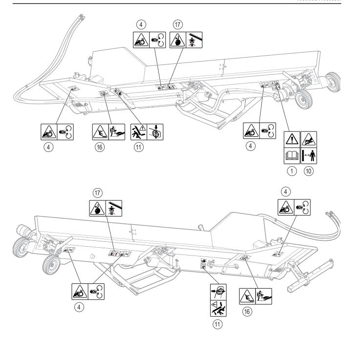
Fig. 6 – 12 ft Conveyor Safety Decal Locations
