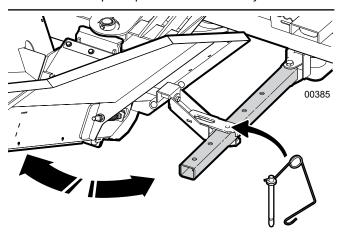
Fig. 36 – Set the Conveyor Angle
