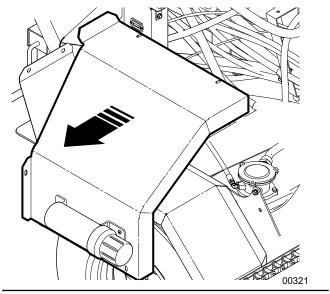
Fig. 79-Hydraulic Oil Reservoir Cover
