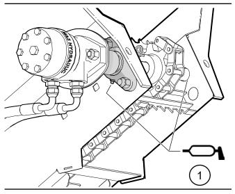
Fig. 97 - 24 ft Conveyor Grease Points
