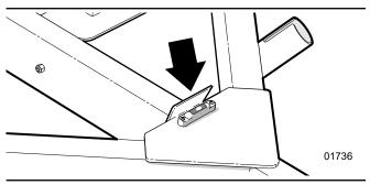
Fig. 21 - Bubble Level on Frame
