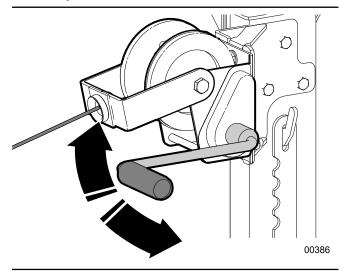
Fig. 14-Conveyor Hand Winch
