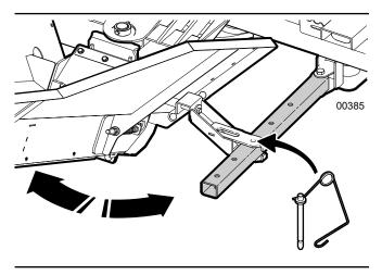
Fig. 15 – Adjust the Conveyor Angle
