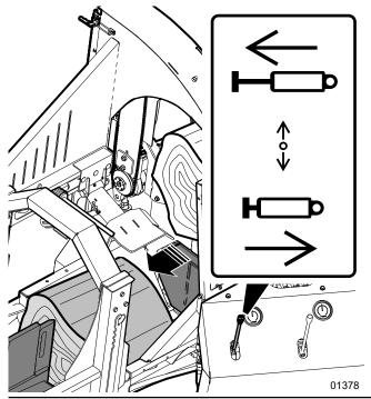
Fig. 63 - Splitter Control Lever
