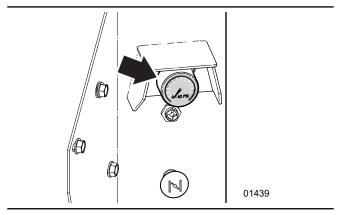
Fig. 78 - Return Filter Bypass Indicator Gauge
