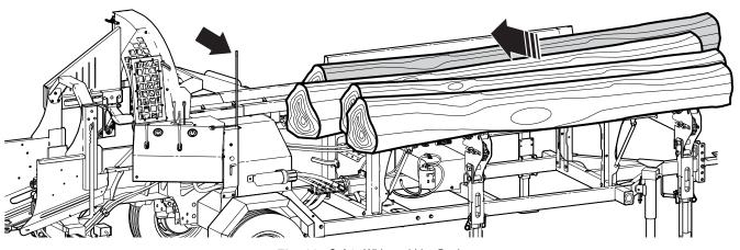
Fig. 68 - Safety Whip and Live Deck
