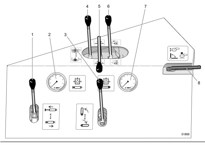
Fig. 20 - Hydraulic Controls
