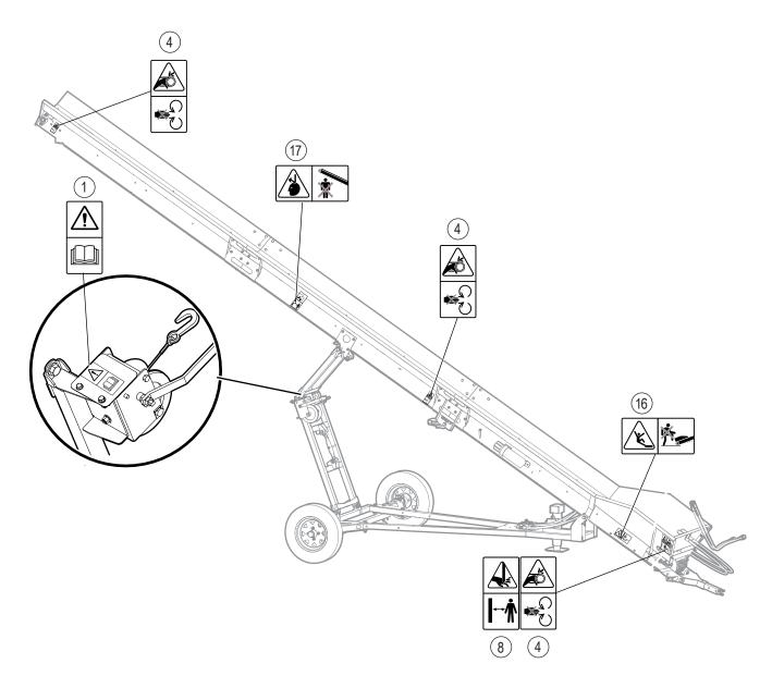
Fig. 7 – 24 ft Conveyor Safety Decal Locations
