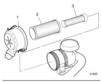
Fig. 83-Cyclonic Engine Air Cleaner
