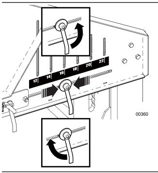
Fig. 29 - Log Stop Guide Lock Handle
