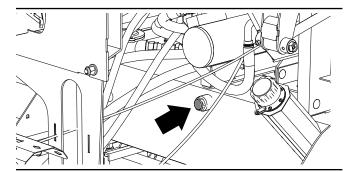
Fig. 40 - Hydraulic Tank Oil Level Check
