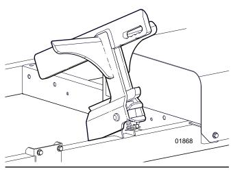
Fig. 65-Splitting Wedge Storage
