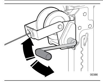
Fig. 35-Conveyor Hand Winch
