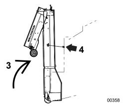
Fig. 74 - 12 ft Conveyor in Transport Position
