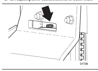
Fig. 58 - Adjusting Screw
