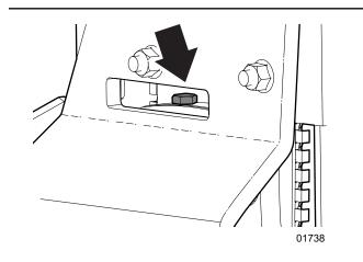
Fig. 88 - Adjusting Screw
