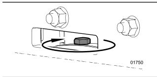
Fig. 89 - Turn Adjusting Screw Clockwise to Increase Chain Tension
