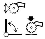
This valve lever clamps / unclamps the Top Roller. The Top Roller can hold a log down and follow its contour as it is cut, then move up out of the way when starting the next log.
