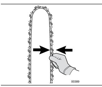
Fig. 43-Check Saw Chain Tension
