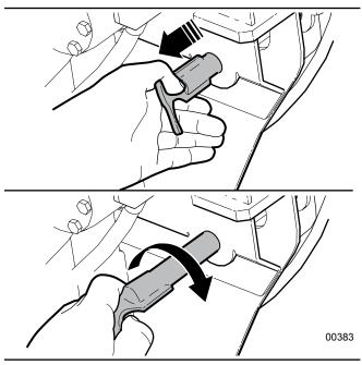
Fig. 23-Live Deck Locking Pins
