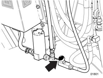
Fig. 60 - Bar Oil Flow Control
