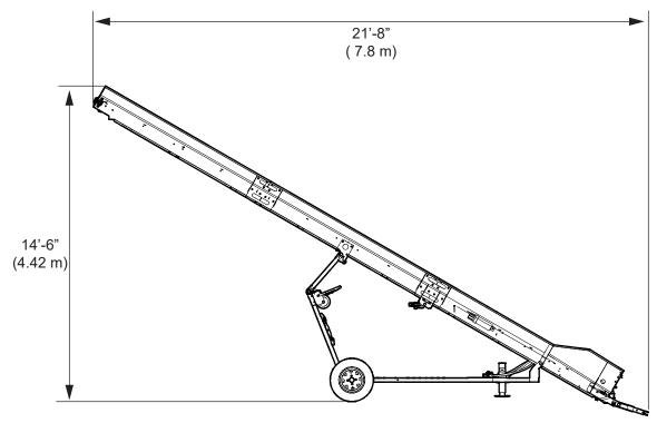
Fig. 103-24 ft Conveyor Dimensions
