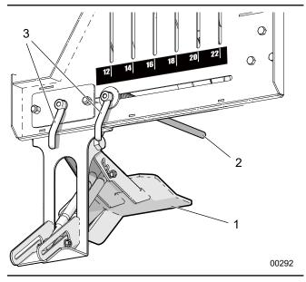
Fig. 27 - Block Dropper and Log Stop Guide
