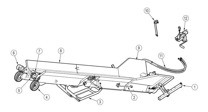
Fig. 18-12 ft Conveyor Components
