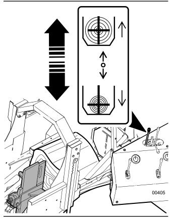
Fig. 61 - Adjust Wedge Height
