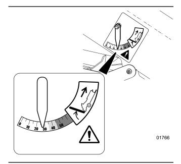
Fig. 34 - Conveyor Angle Indicator
