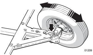
Fig. 37 - Rotating the Conveyor Wheels
