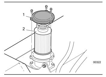
Fig. 80 - Hydraulic Oil Filter Element
