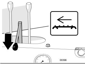
Fig. 46-Infeed Conveyor Control Valve
