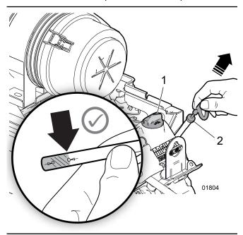
Fig. 39 - Checking Engine Oil Level
