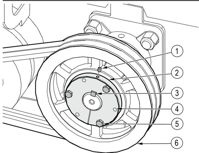
**Figure 43**—Rotor sheave
