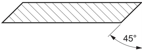
**Figure 45**—Sharpen rotor knives to a 45° angle
