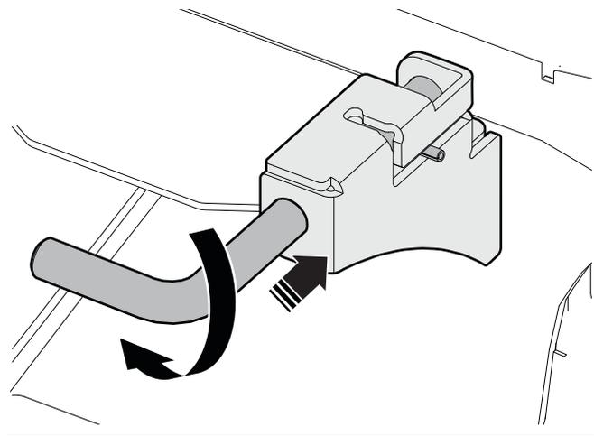
Figure 24—Engage the rotor lock
