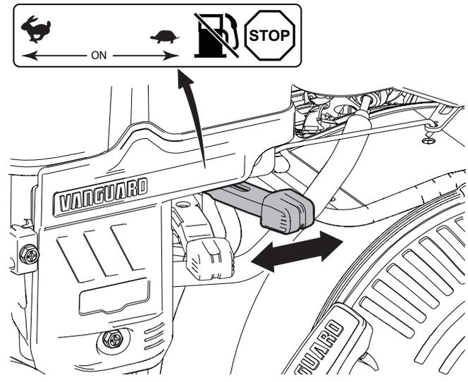
Figure 9—Engine throttle control and fuel shutoff
