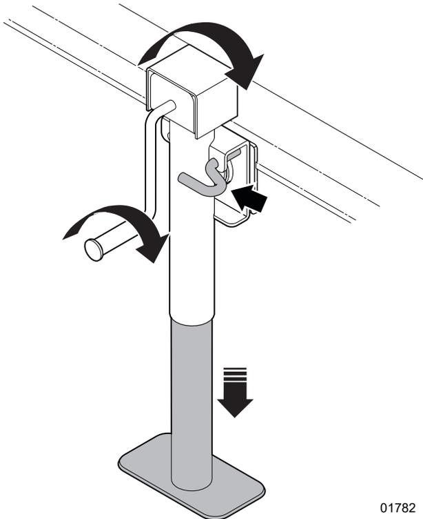
**Figure 28**– Trailer jack in the lowered position
