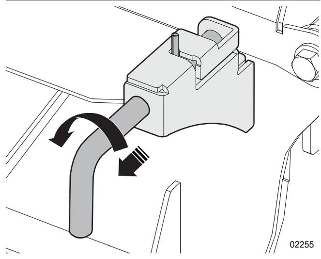
Figure 16—Disengaged position
