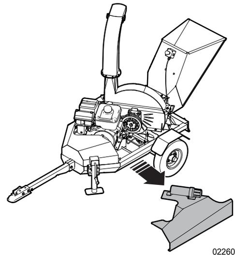
Figure 35—Remove the drive-belt guard
