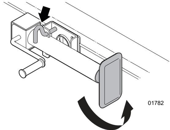
**Figure 29**– Trailer jack in the stowed position
