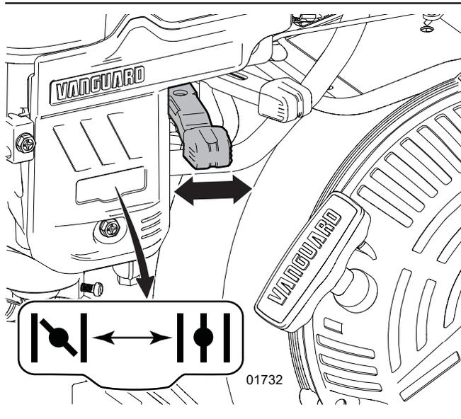
Figure 10—Engine choke control
