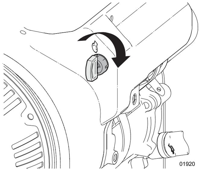
Figure 11—Ignition switch control
