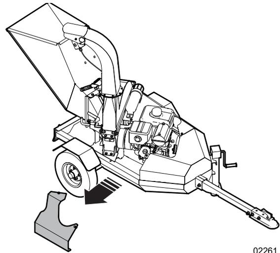
Figure 34—Remove the engine guard
