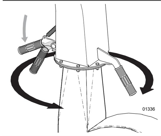
Figure 13—Turn the discharge chute
