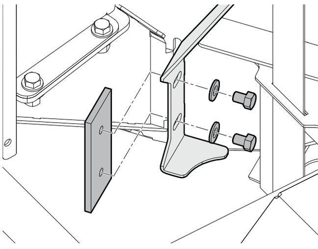
Figure 46—Install a ledger knife
