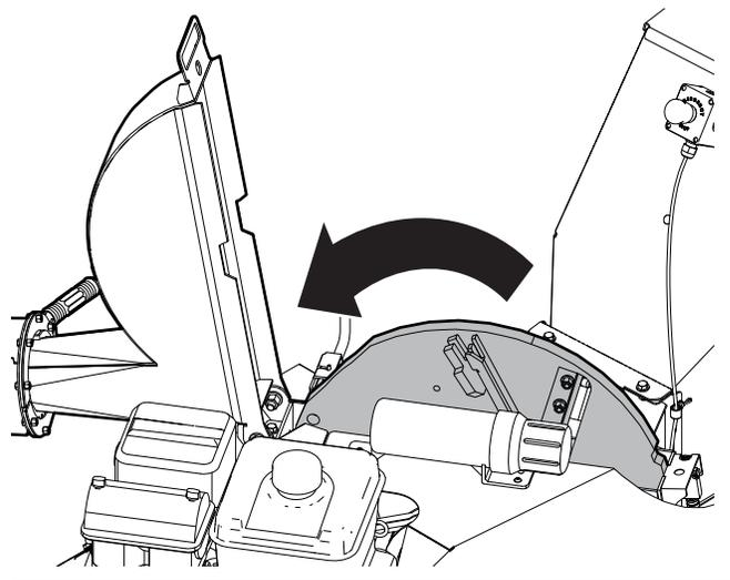
Figure 23—Open the upper rotor housing
