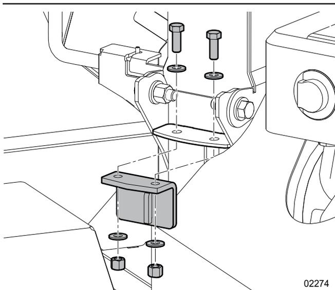
**Figure 49**—Install a twig breaker
