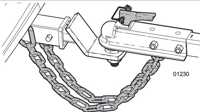
**Figure 27**—Ball-mount hitch connection
