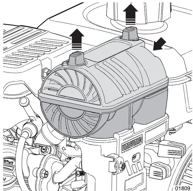
**Figure 33**—Engine air filter
