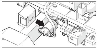
Figure 29-Hydraulic fluid filter (WXR740)
