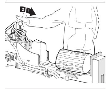
Figure 20-High speed position (2), High power position (1)
