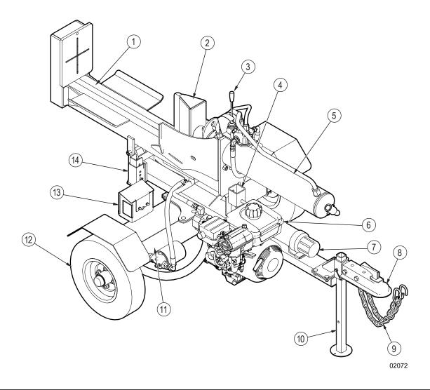
Figure 4-WXR740, WXR740L log splitter components
