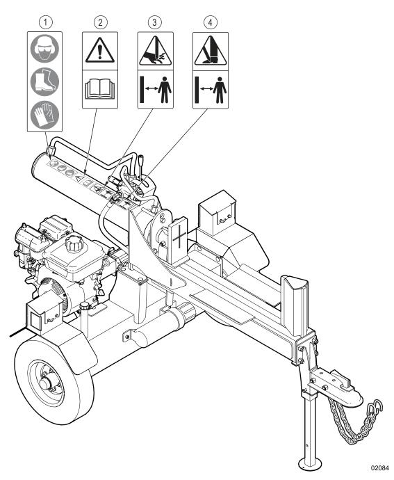
Figure 2-Safety decal locations (typical for all WX700 series models)
