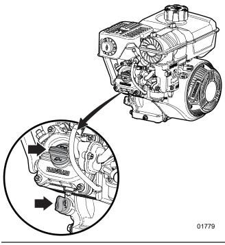
Figure 12-Engine oil-fill locations
