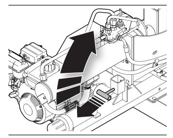
Figure 22-Rotate the splitter to vertical
