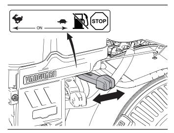
Figure 5-Engine throttle control and fuel shutoff
