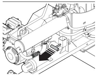
Figure 24-Lock pin is fully engaged (WXR740)
