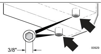
Figure 27 – Hydraulic tank drain plugs
