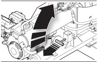
Figure 17-Rotate the WXR740 or WXR740L to vertical
