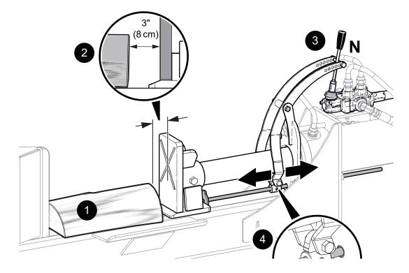
Figure 10-Set the stroke limiter accessory
