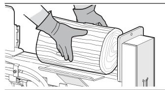
Figure 18–Correct log placement
