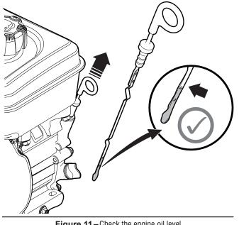
Figure 11 – Check the engine oil level
