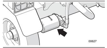
Figure 28-Hydraulic fluid filter (WXR720)
