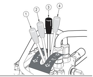
Figure 19-Splitter-control valve
