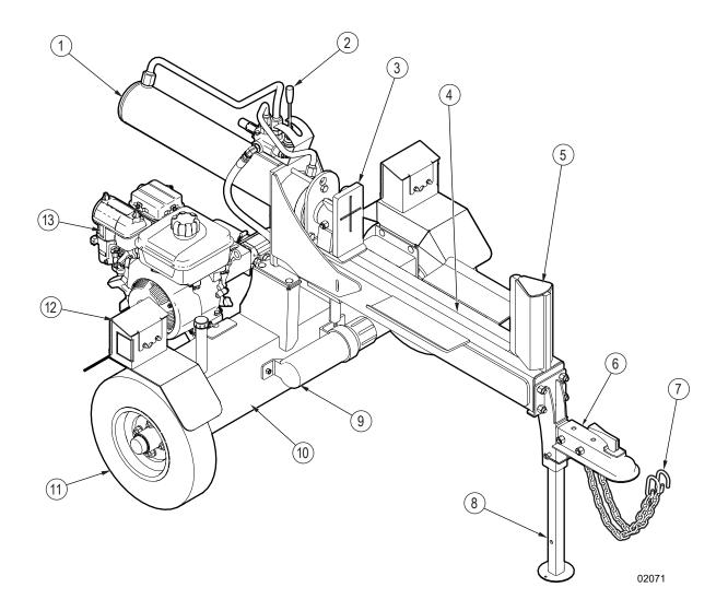
Figure 3-WXR720, WXR720L log splitter components
