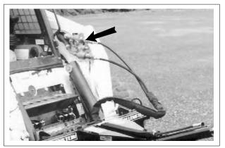
Fig. 2 HYDRAULIC OUTLETS (typical)
