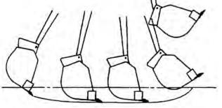
Fig. 11 DIGGING WITH BOOM
