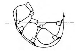
Fig. 12 DIGGING WITH BUCKET
