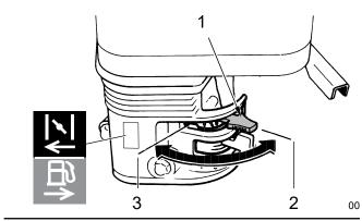
Fig. 6-Choke Lever
