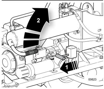
Fig. 28-Rotate Splitter to Vertical
