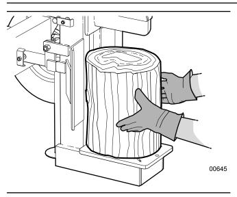
Fig. 29-Correct Log Placement—Vertical
