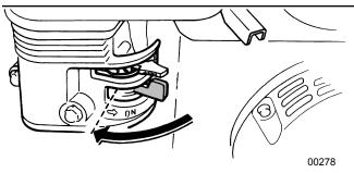
Fig. 32-Fuel Valve OFF
