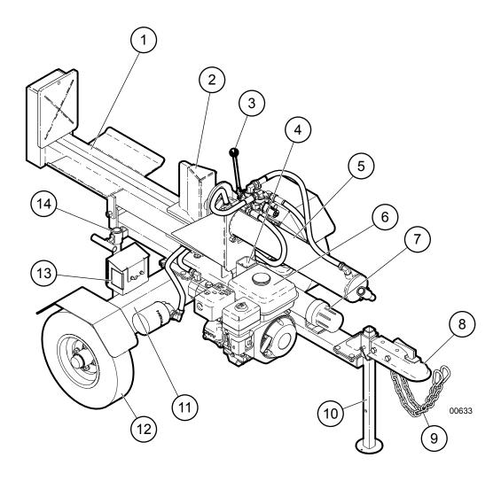
Fig. 3-WX540, WX540L Wood Splitter Components
