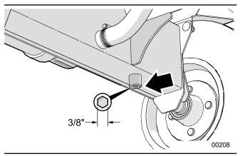
Fig. 35-Hydraulic Tank Drain Plug
