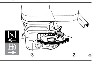
Fig. 19-Choke Lever
