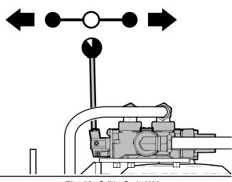
Fig. 10-Splitter Control Valve
