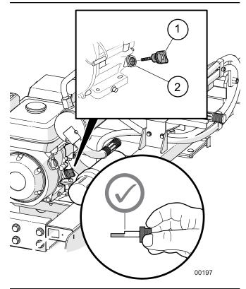
Fig. 15-Engine Oil Level check
