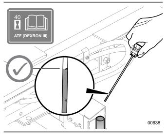
Fig. 16–Hydraulic Tank Oil Level Dipstick
