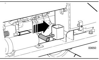
Fig. 31 – Lock Pin Fully Engaged
