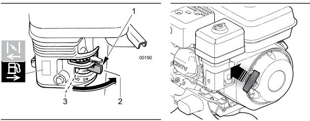
Fig. 7-Fuel Valve Lever
