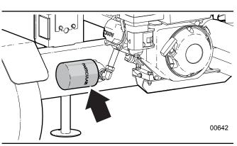
Fig. 36-Hydraulic Oil filter
