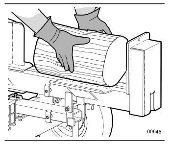
Fig. 24-Correct Log Placement-Horizontal
