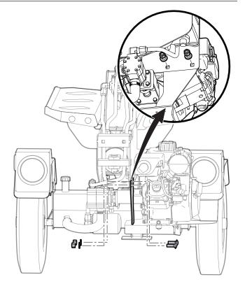
Align the bolt holes on license plate light assembly (4) with the bolt holes on the rear machine frame. Install the fasteners that were removed in step 9.
