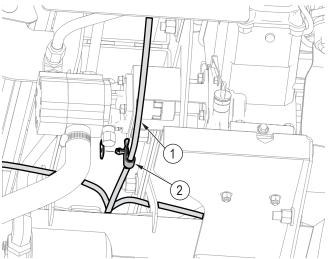
Install the two middle cable clamps (2) into the two machine frame cable-clamp mount holes.
