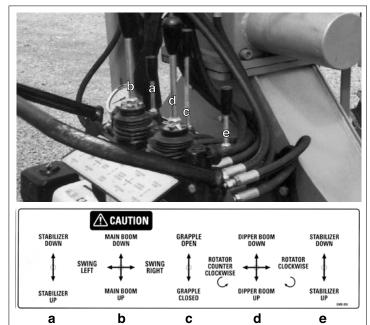
Fig. 3 HYDRAULIC CONTROLS
