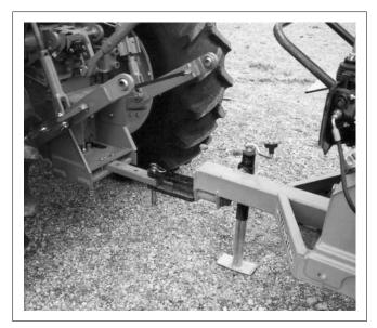
Fig. 4 DRAWBAR PIN AND RETAINER
