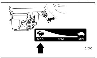
Fig. 24-Move throttle setting to MAX
