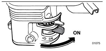
Fig. 19-Fuel valve Lever
