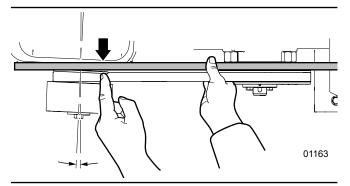
Fig. 36-Engine Mount Misalignment
