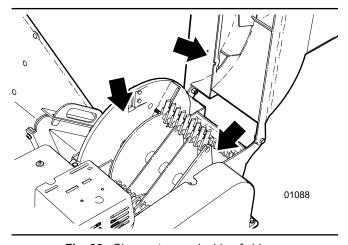
Fig. 30 - Clear out areas inside of chipper
