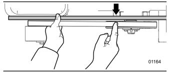
Fig. 38-Rotor Sheave Misalignment
