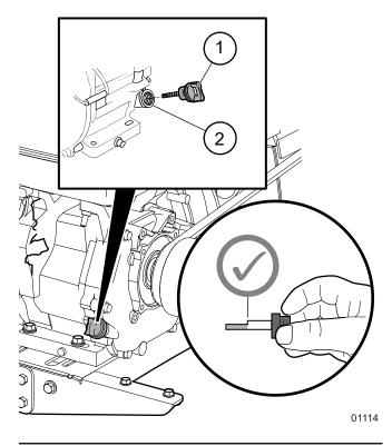
Fig. 18-Engine Oil Level check
