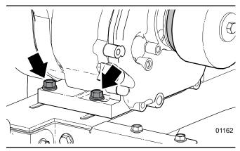
Fig. 37 - Engine Mount Bolts
