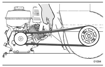
Fig. 34-Rotor drive belt tension
