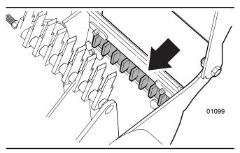
Fig. 43-Chop Block in Rotor Housing
