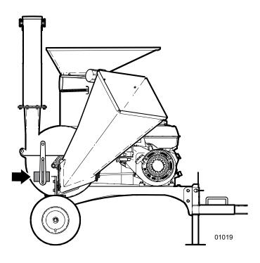
Fig. 1-Serial Number Plate Location
