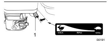
Fig. 21 - Engine Throttle
