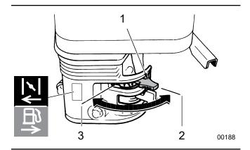
Fig. 20 - Choke Lever
