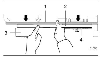
Fig. 35-Drive Belt alignment
