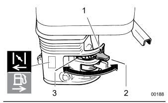
Fig. 8-Choke Lever
