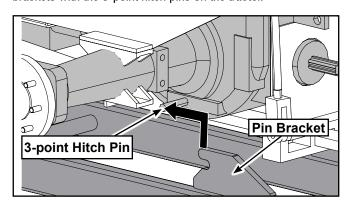
Carefully back up the tractor until the pins engage the pin brackets.
