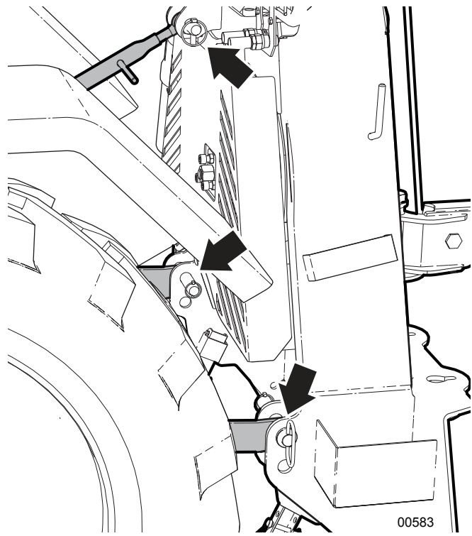
Figure 35 —Three-point hitch attachment locations
