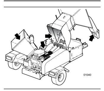
Fig. 23 – Clear out areas inside of chipper
