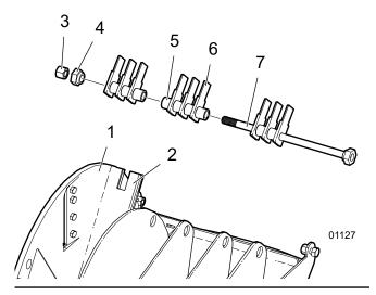
Fig. 43-Rotor Assembly
