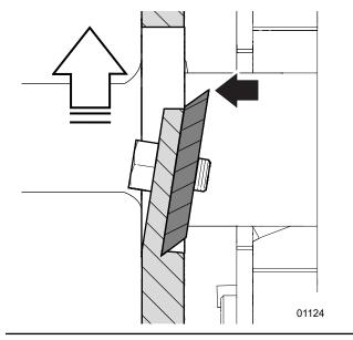
Fig. 37 - Rotor blade leading edge outward
