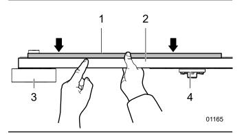
Fig. 30 - Drive Belt Alignment
