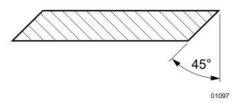
Fig. 36-Sharpen Blade at 45° angle
