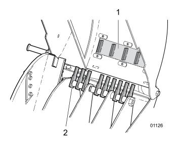
Fig. 42-Chop Block in Rotor Housing
