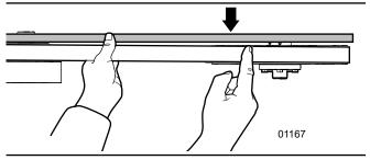
Fig. 34-Rotor Sheave Misalignment
