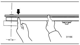
Fig. 31 - Engine Mount Misalignment
