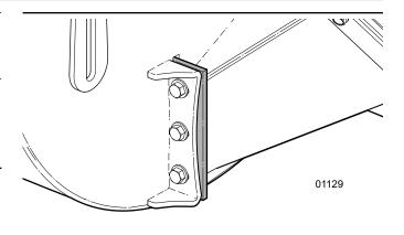
Fig. 38-Ledger knife inside lower rotor housing
