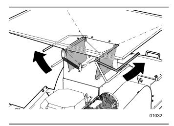
Fig. 12-BXMT4224 Feed Gate Levers
