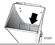
Fig. 20-Feed Hopper Safety Curtain
