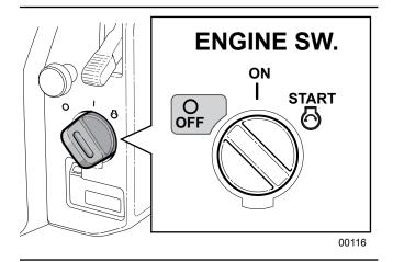
Fig. 9-Engine Start Switch
