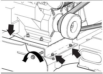
Fig. 28-Drive Belt Tension Adjuster Bolt
