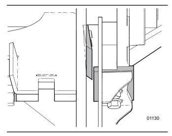
Fig. 39 - Checking ledger knife clearance
