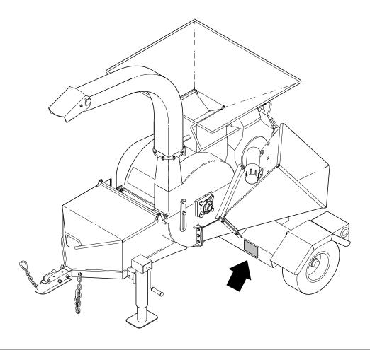
Fig. 1-Serial Number Plate Location (Typical)
