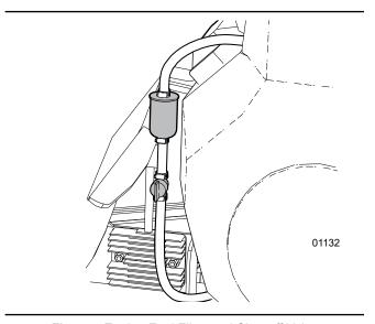
Fig. 45-Engine Fuel Filter and Shut-off Valve
