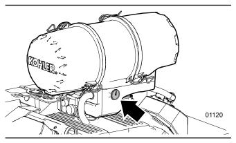
Fig. 26-BXMT4238 Air Filter Restriction indicator
