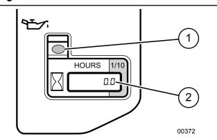
Fig. 10-Engine Hours and Oil Level Alert
