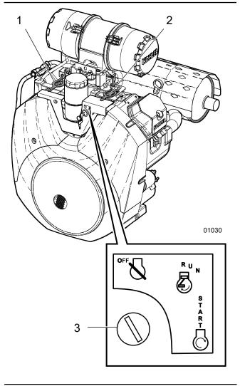
Fig. 11 - Engine Controls
