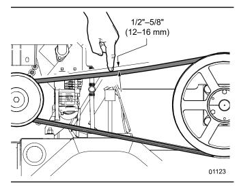
Fig. 29-Rotor drive belt tension
