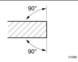
Fig. 41 - Sharpening Ledger Knife
