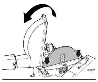
Fig. 57-Open Upper Rotor Housing
