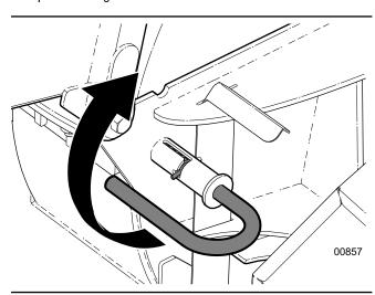
Fig. 34-Rotor Unlocked Position
