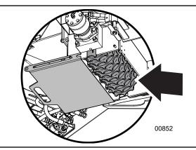
Fig. 59 - Lower Roller Clean-out Tray
