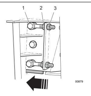
Fig. 78-Adjusting Ledger Knife
