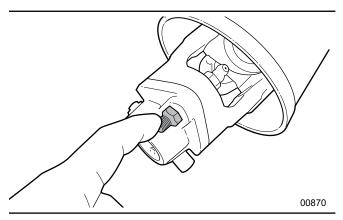
Fig. 71-PTO Shear Pin
