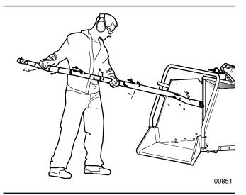
Fig. 55-Stand to Side of Feed Table
