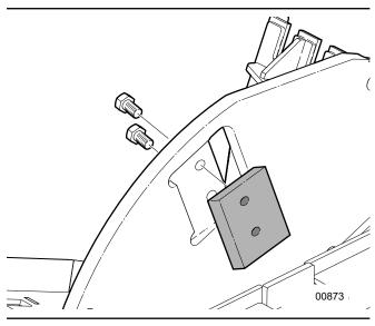
Fig. 73-Changing rotor blade
