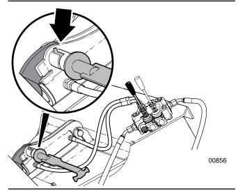
Fig. 44-Cylinder Locking Pin in Place
