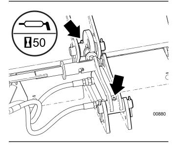
Fig. 67-Hydraulic Feed Roller Lift Cylinder
