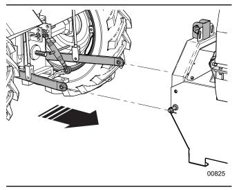
Fig. 9-Back up in line with the chipper
