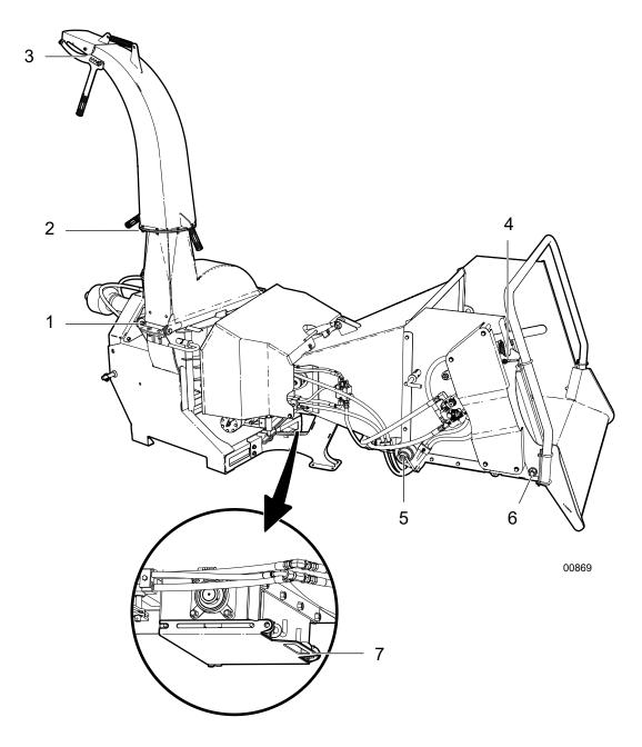
Fig. 69-Grease Hinges and Pivot Points
