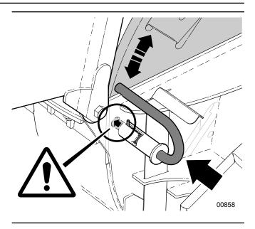
Fig. 35-Rotor Locked Position
