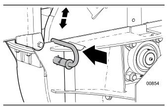
Fig. 58 - Engage Rotor Lock
