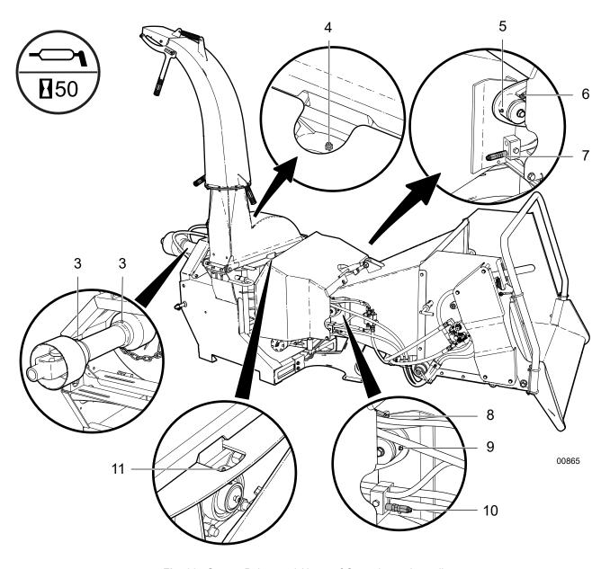
Fig. 66 - Grease Points - 50 Hours of Operation or Annually
