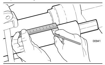
Fig. 13-Place mark to cut plastic tube
