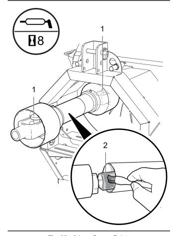
Fig. 65 - 8-hour Grease Points
