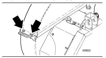
Fig. 56-Rotor Housing Flange Bolts
