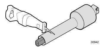
Fig. 14-Cut plastic tube at the mark
