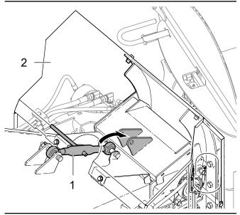
Fig. 60 - Connect Toplink to Bridge
