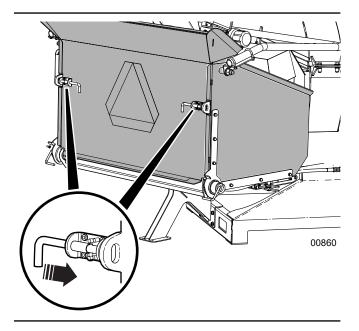
Fig. 63-Feed Table in Stowed Position
