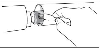
Fig. 16-Grease the inner tube
