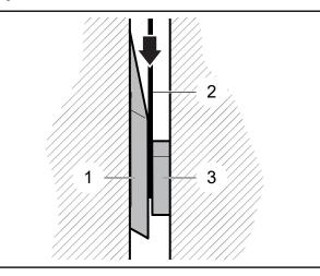
Fig. 77 - Checking ledger knife clearance
