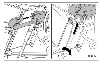
Fig. 83-Locking Pin on BX102RP Models
