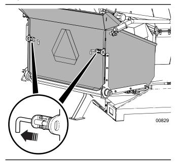
Fig. 49-Feed Table in Stowed Position
