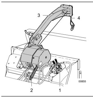
Fig. 46-Hydraulic Winch
