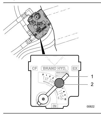
Fig. 32-Flow Control Valve
