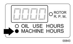
Fig. 40 - Machine Hours Screen
