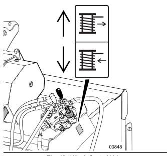
Fig. 48-Winch Control Valve
