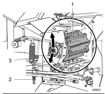
Fig. 33-Cutaway View to see Upper Roller
