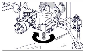
Fig. 80 - Tension Spring hex Nuts
