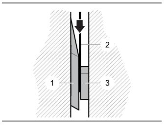
Fig. 26 - Checking ledger knife clearance
