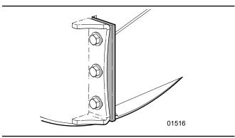
Fig. 23 – Ledger Knife inside Lower Rotor Housing
