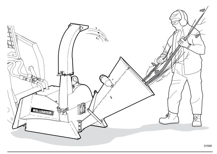
Fig. 19 - Chipper Setup to Operate
