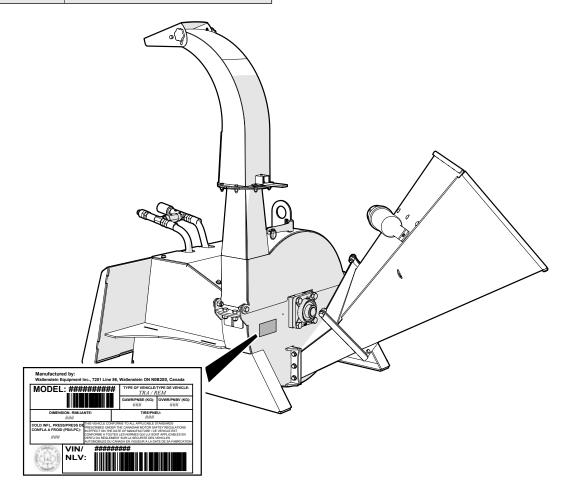
Fig. 1 – Serial Number Plate Location
