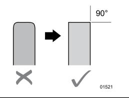
Fig. 24-Ledger Knife Sharpness
