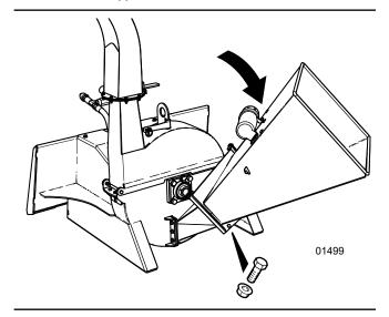
Fig. 11 – Feed Hopper Lowered
