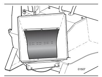
Fig. 13-Feed Hopper Safety Curtain
