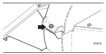
Fig. 16-Rotor Housing Flange Bolt
