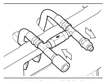
Fig. 8 – Hydraulic Connections—3/4" Flat Face Couplers
