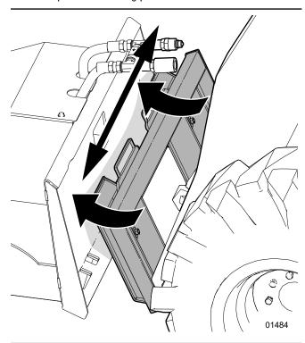
Fig. 6-Align Skid Steer with Mounting Plate
