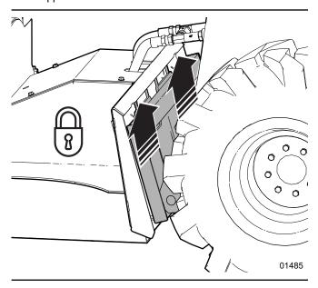
Fig. 7-Insert Skid Steer Face Plate into Chipper Mount
