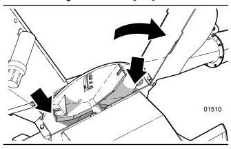
Fig. 17 - Open Upper Rotor Housing
