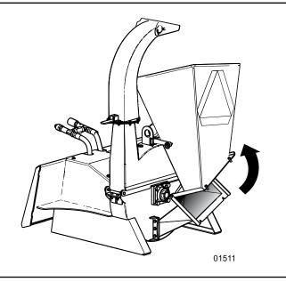
Fig. 15-Open Lower Feed Hopper
