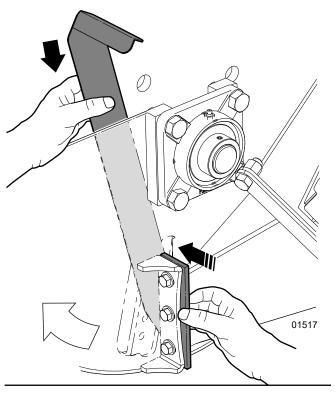
Fig. 25 - Checking Ledger Knife Clearance with Ledger Setting Gauge
