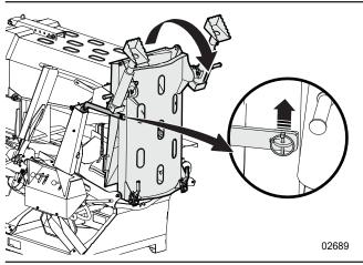
Figure 13–Disconnect the bar latch and unfold the log-loader and lead-in chutes
