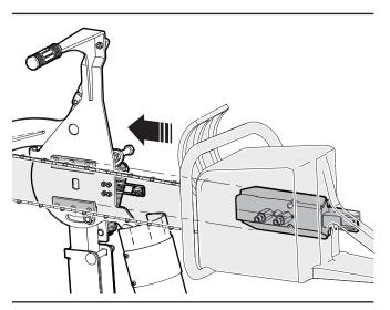
Figure 23-Put the chainsaw into the chainsaw holder
