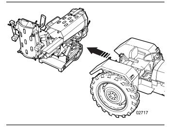
Figure 45-Align the tractor with the machine
