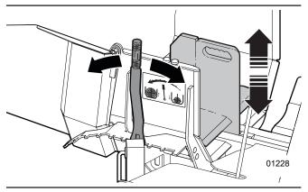
Figure 9-Splitting-wedge height adjustment
