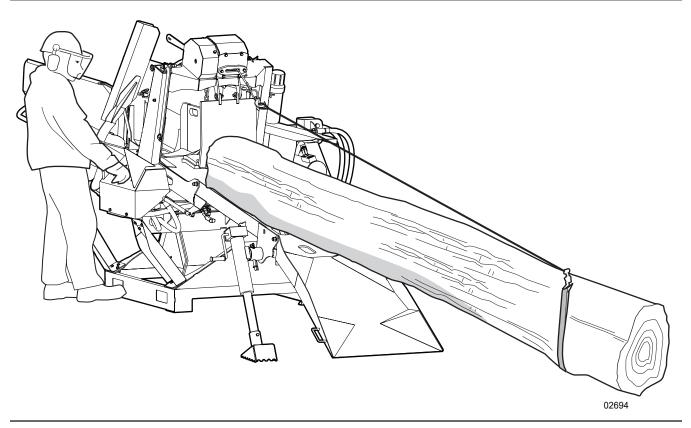
Figure 31-Position the log in the machine
