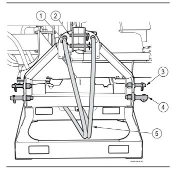
Figure 44-Machine three-point hitch connections (WP245 shown)
