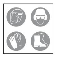
**Information labels** are usually pictorial with a white background and the number of panels can be different. This type of gives information to the operator or shows the operation of a control.
