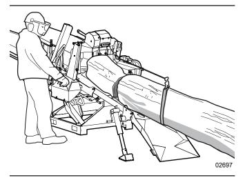
Figure 38-Use the next log to push the current log
