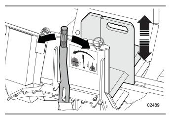
Figure 19-Set the splitting-wedge height
