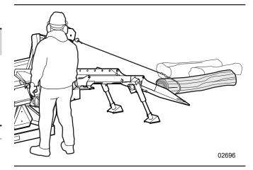
Figure 29-Pull the first log to the machine
