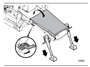
Figure 14–Engage the toggle-clamp latches and unfold the lead-in chute
