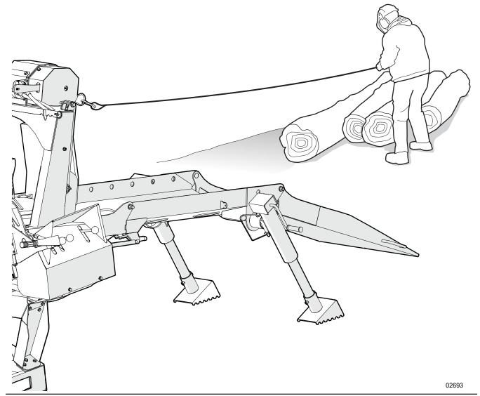
Figure 28-Pull the winch rope out to the log
