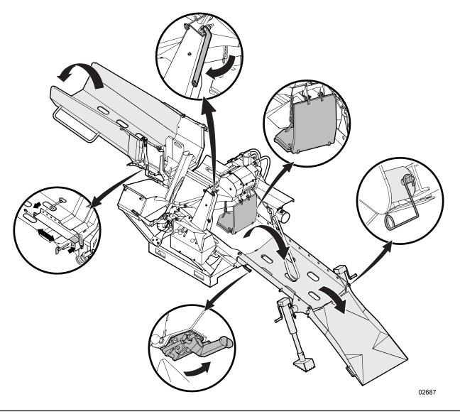
Figure 11 - Machine setup (WP245 shown)
