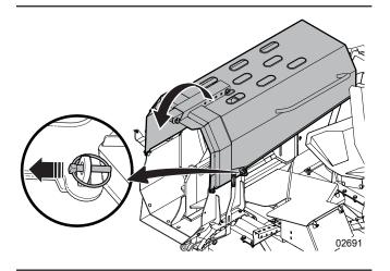
Figure 16–Splitter chute linchpin and latch tab
