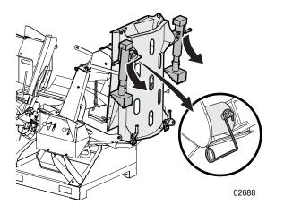
Figure 12-Extend the support jacks
