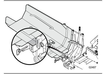
Figure 17 – Install the hitch pin through the splitter chute and splitting cradle bracket
