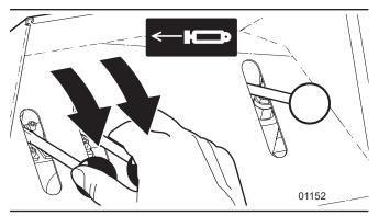
Figure 35-Push the two splitter cylinder control levers down
