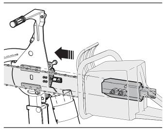
Figure 32–Put the chainsaw into the holder
