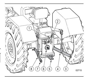
Figure 43-Tractor three-point hitch connections (example)
