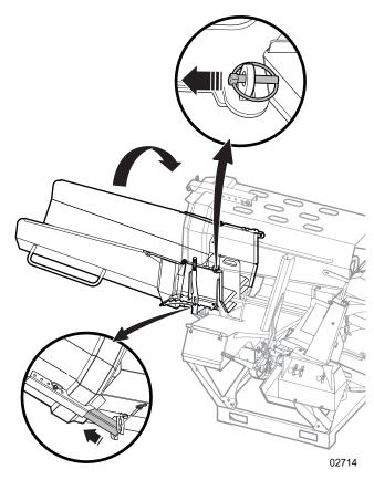
Figure 41 - Fold the splitter chute
