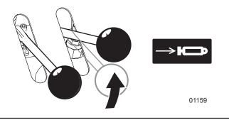
Figure 36-The push block retracts automatically
