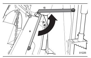
Figure 40–Use the latch bar and linchpin to hold the chutes in the folded position
