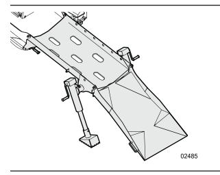
Figure 15-The log-loader and lead-in chutes unfolded
