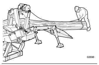
Figure 30-Move the winch strap
