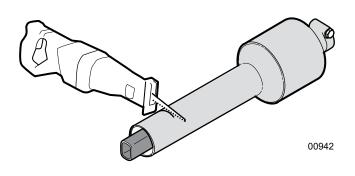
Fig. 14–Cut plastic tube at the mark
