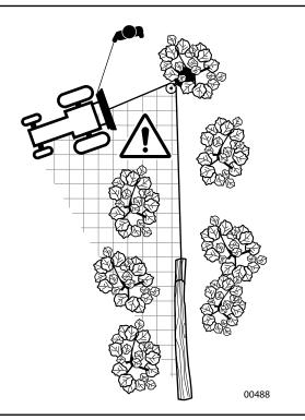
Fig. 40-Using Snatch Block or Self-releasing Pulley
