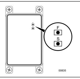
Fig. 38-Receiver Function and Select Buttons
