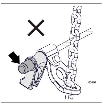
Fig. 25-Incorrect use of Forged End
