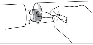
**Fig. 16**–Grease the inner tube
