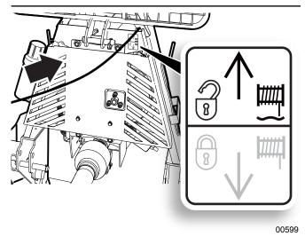
Fig. 45–Unlock Winch Drum
