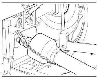
Fig. 9-PTO Shaft Installed
