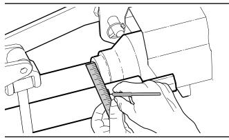
Fig. 12-Transferring the mark
