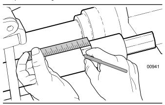
Fig. 13-Place mark to cut plastic tube
