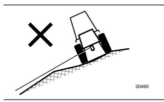
Fig. 41 – Never Winch from the Side on a Slope
