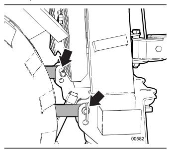
Fig. 7-Hitch Pins Installed
