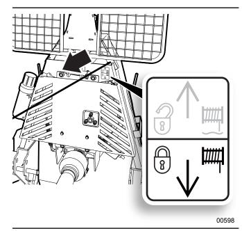
Fig. 44-Winch Drum Lock
