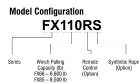
FX110 - 11,000 lb FX140 - 14,000 lb Safe, efficient and trouble-free operation of this Wallenstein product requires that anyone using or maintaining the machine reads and understands the Safety, Operation, Maintenance information contained within this Operator's Manual.
