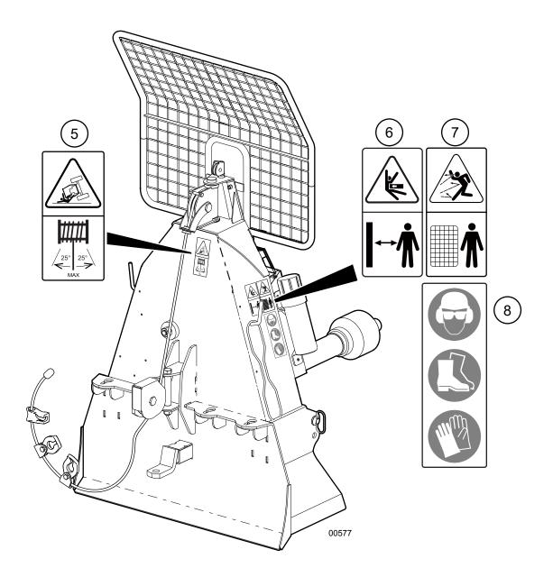
Fig. 3-FX-Series Safety Decal Placement
