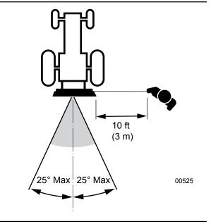
Fig. 39-Safe Winch Angle
