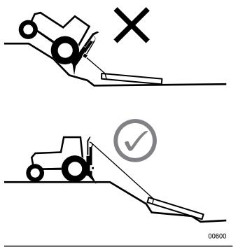
Fig. 46-Winch Log over Rough Ground
