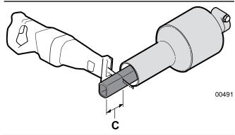
Fig. 20-Cut off the Length C from both PTO Shaft halves
