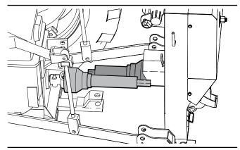
Fig. 11 – Lift shaft ends up parallel
