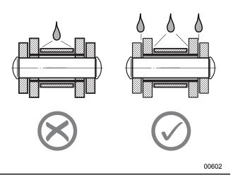
Fig. 48-Proper Roller Chain Lubrication
