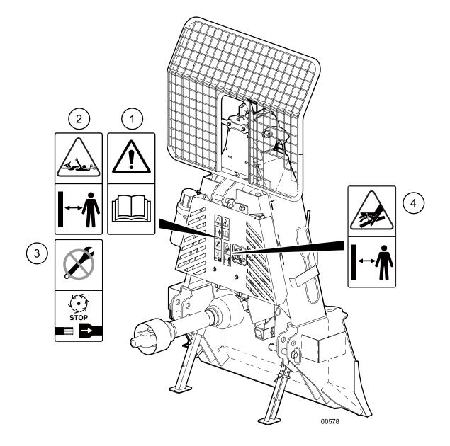
Fig. 2-FX-Series Safety Decal Placement
