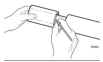
Fig. 15-Marking steel tube.
