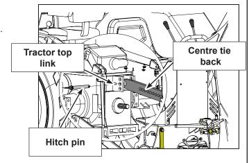
5. Assemble the two tie back bar sides to backhoe seat brace / top link with a bolt. (not included)
