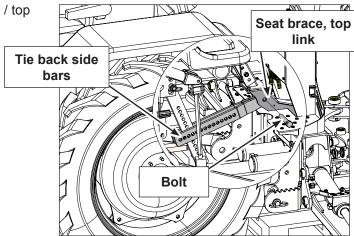
Start the tractor, raise the lower link arms so the backhoe bottom is approximately 13" (330mm) from the ground. Use the backhoe boom and stabilizers to align the centre and side tie back bars. Ensure the backhoe is straight and level.
