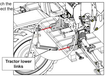
3. Find the centre tie back bushing (1" id) and check that it fits on the tractors top link, if the bushing is too wide then it will have to be cut to fit.
