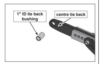
4. Attach the centre tie back and bushing to the tractor top link. using a hitch pin.
